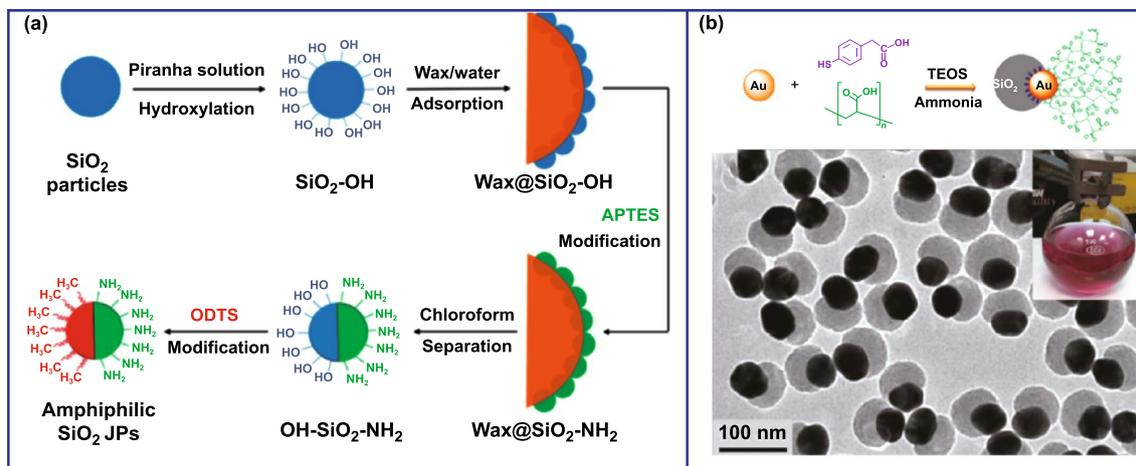
**Fig. 8** Preparation of various asymmetric silica-based nanoparticles. **a** Preparation of amphiphilic Janus silica particles by Pickering emulsion. Reproduced with permission from Ref. [100]. Copyright 2015, American Chemical Society. **b** Preparation of Janus Au-SiO<sub>2</sub> nanoparticles by selective modification. Reproduced with permission from Ref. [106]. Copyright 2010, American Chemical Society
