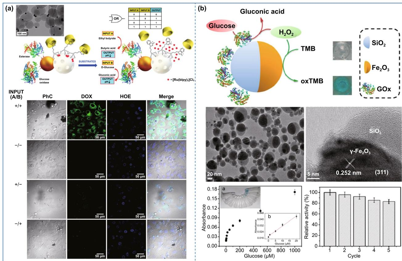
**Fig. 14** Application of asymmetric structure in others. **a** Application of Janus gold-mesoporous silica nanoparticles in logic gate. Reproduced with permission from Ref. [149]. Copyright 2014, American Chemical Society. **b** Application of Janus particles in sensors. Reproduced with permission from Ref. [151]. Copyright 2015, American Chemical Society
