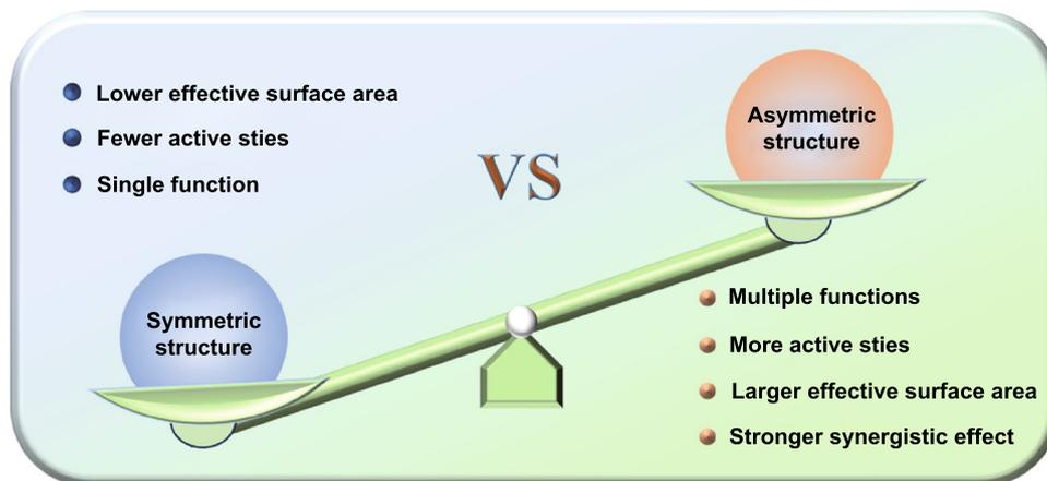
**Fig. 2** Comparisons of advantages and disadvantages of symmetric and asymmetrical structures
