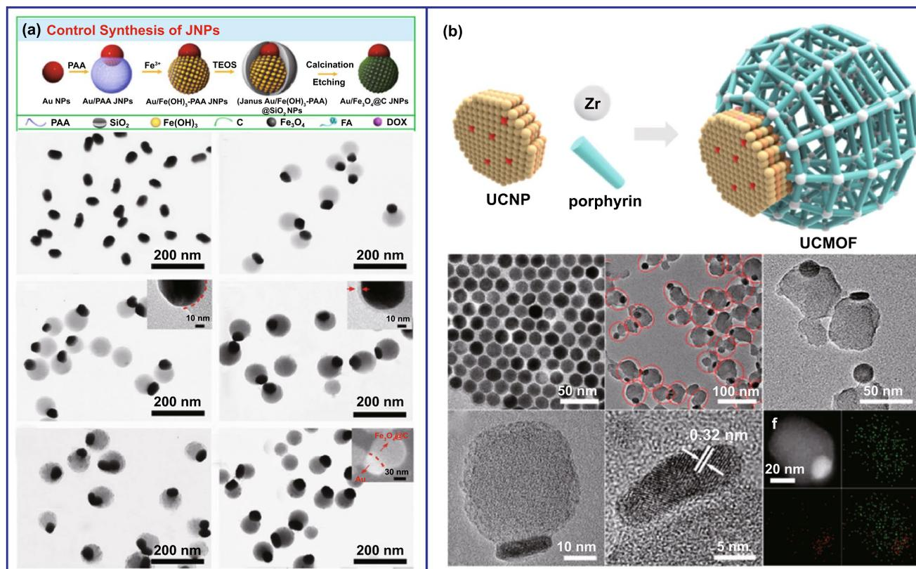
**Fig. 5** Preparation of various asymmetric polymer- and MOF-based nanoparticles. **a** Preparation of Au/Fe<sub>3</sub>O<sub>4</sub>@C Janus nanoparticles by controlling the surface interfacial energy. Reproduced with permission from Ref. [51]. Copyright 2017, Wiley–VCH. **b** Fabrication of Janus structured MOF-UCNPs by selectively modifying the surface. Reproduced with permission from Ref. [54]. Copyright 2017, American Chemical Society
