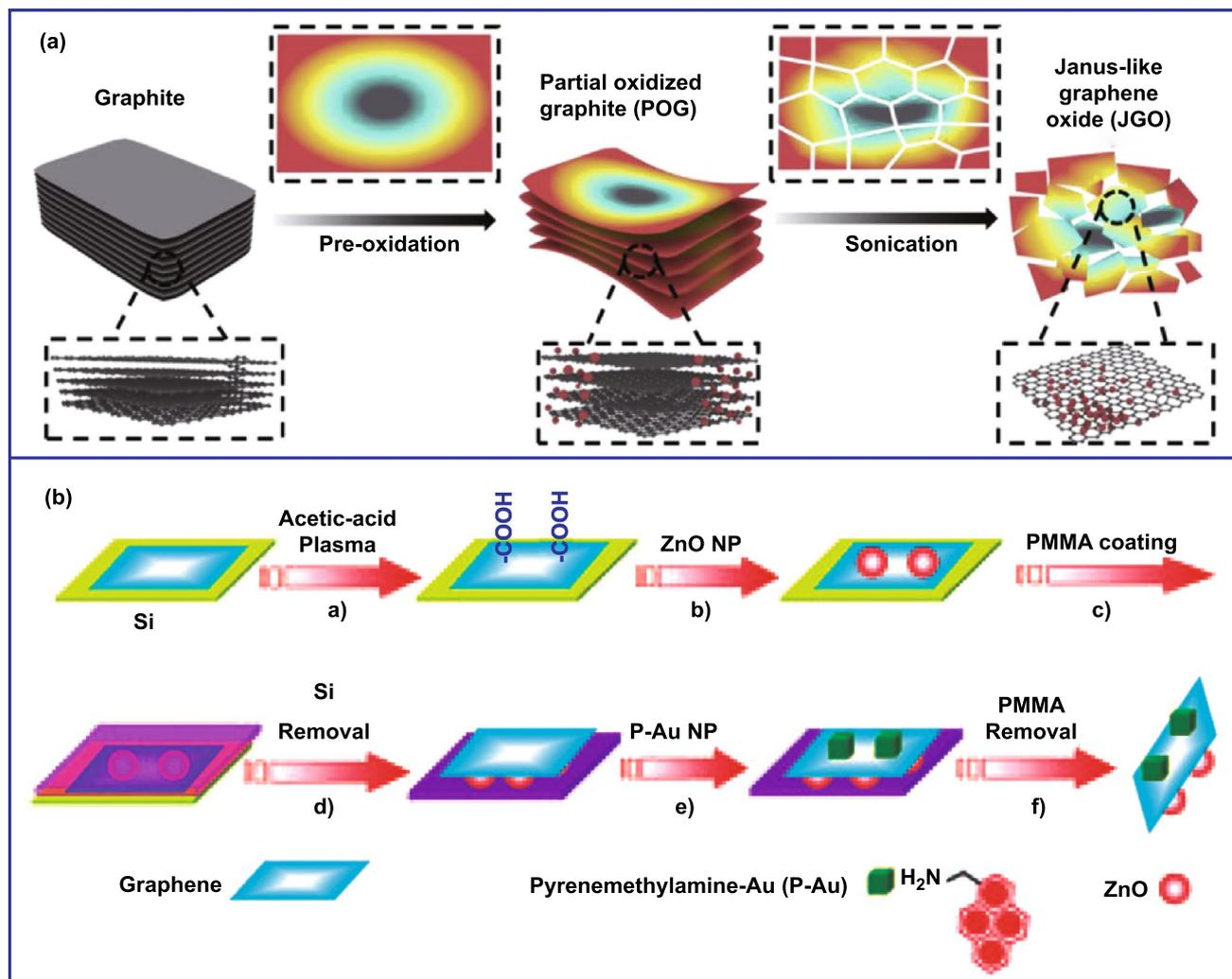
**Fig. 6** Preparation of various asymmetric carbon-based nanomaterials. **a** Preparation of novel asymmetric structure along the faces of the sheets. Reproduced with permission from Ref. [69]. Copyright 2020, Elsevier B.V. **b** Fabrication of Janus structured ZnO-graphene-Au composite materials by selectively modifying the surface. Reproduced with permission from Ref. [70]. Copyright 2011, Wiley-VCH
