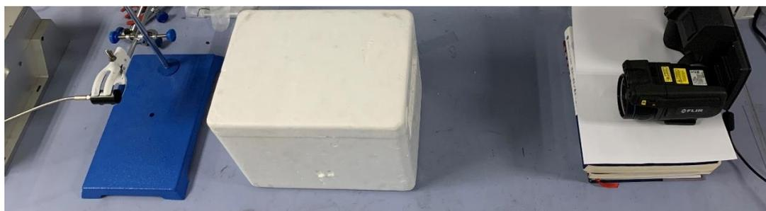
**Fig. S15** The digital photo of the test system used to investigate light-to-heat conversion capability including a laser light generating the powerful irradiation (left), an infrared (IR) camera recording the surface temperature of the sample (right) and some liquid nitrogen placed in the foam chamber creating a low-temperature environment (middle)
