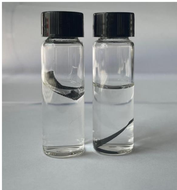
**Fig. S3** Digital photo of primary carbon cloth (left) and treated carbon cloth (right) submerged in water
