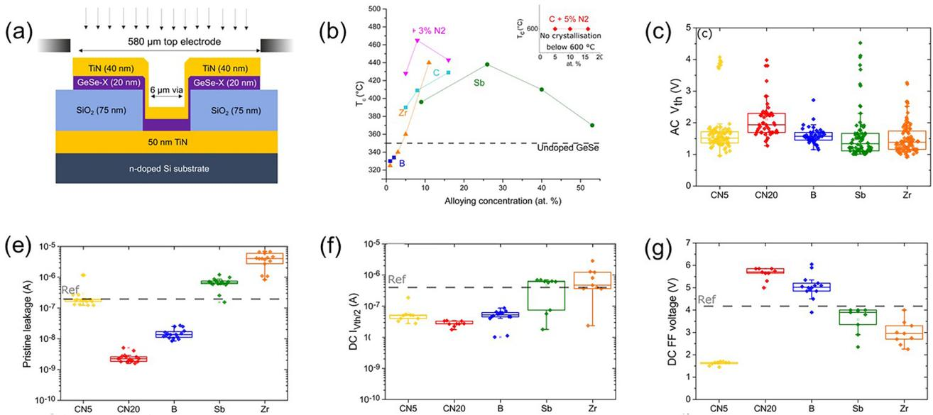
**Fig. 8** C/Sb/B/N/Zr-doped GeSe OTS selectors. **a** Device structure with  $6\ \mu\text{m}$  size. **b** Crystallization temperature  $T_c$ . **c** Alternating current (AC)  $V_{\text{th}}$ . **e** Pristine leakage at  $1\ \text{V}/2\ \text{V}$ . **f**  $I_{\text{off}}$ . **g**  $V_{\text{ff}}$  voltage. Adapted with permission from [49]. Copyright 2021, AIP Publishing
