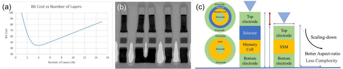
**Fig. 29** a The bit cost versus number of layers [148]. b An example image of leaning and the resulting bridges in 3D XPoint structure. Adapted with permission from [151]. Copyright 2022, IEEE. c Concept of SSM (Self-Selecting Memory) in vertical and plane structure
