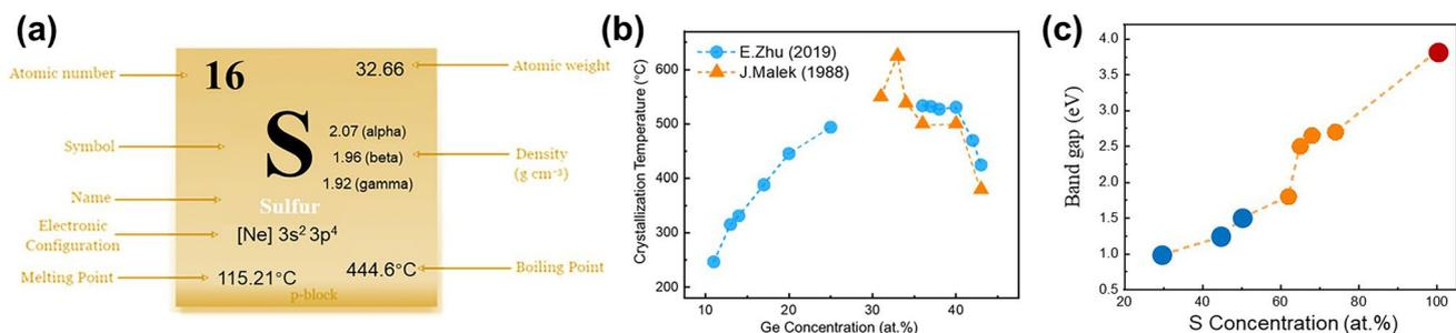
**Fig. 17** Elemental S and Ge-S properties. **a** Element sulfur's properties. **b** Crystallization temperatures and **c** the mobility gap of Ge-S alloys [81–83]
