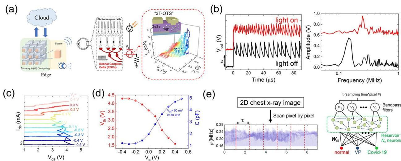
**Fig. 34** 3 T-OTS device as an artificial RGC. **a** Concept of edge- and cloud-computation, the diagram of RGC and an artificial RGC. **b** Response waveform of an artificial RGC with/without illumination, and the FFT spectra. **c** Variations of  $V_{th}$  under the modulation of  $V_g$ . **d**  $V_{th}$  and  $C$  versus  $V_g$ . **e** Classification of chest X-ray images between normal and other virus [189]. Adapted with permission from [189]. Copyright 2022, American Chemical Society
