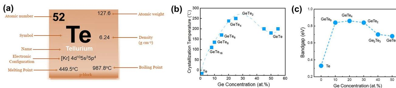
**Fig. 10** Elemental Te and Ge–Te properties. **a** Element tellurium's properties. **b** Crystallization temperatures ( $T_c$ ) [56] (Adapted with permission from [56]. Copyright 1986, AIP Publishing) and **c** the mobility gap [57] (Adapted with permission from [57]. Copyright 1974, Elsevier) of Ge–Te alloys, respectively
