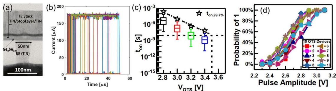
**Fig. 35** Ge–Se-based true random number generator. **a** Device structure with 50-nm plug. **b** Distribution of  $t_{delay-on}$  at 2.8 V. **c** Distribution of  $t_{on}$  at different biases. **d** Occurrence rate of “1” at different pulse amplitudes measured in 10 devices [196]. Adapted with permission from [196]. Copyright 2021, IEEE
