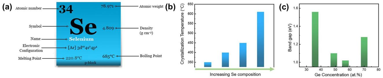
**Fig. 5** Elemental Se and Ge–Se properties. **a** Element selenium’s properties. **b** Crystallization temperatures ( $T_c$ ) [38] and **c** mobility gap of Ge–Se alloys [39, 40]. Adapted with permission from [39]. Copyright 2011, IOP Publishing
