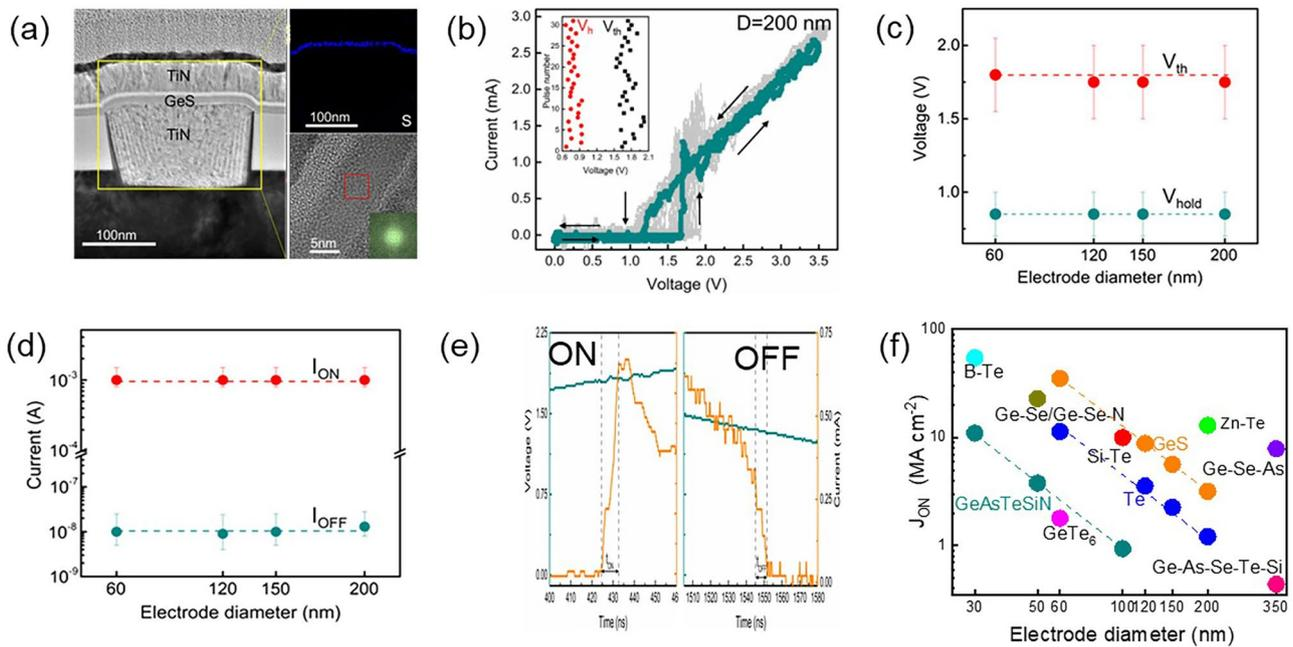
**Fig. 19** GeS OTS device with TiN electrodes. **a** Device structure with 60–200-nm plug. **b** AC  $I$ – $V$  sweeps. **c**, **d**  $V_{th}$ ,  $V_{hold}$ ,  $I_{on}$  and  $I_{off}$  dependence on the electrode size. **e** On/Off speed; **f** Comparison of the  $J_{on}$  of the GeS OTS cell with other Te- and Se-based selectors [95]. Adapted with permission from [95]. Copyright 2021, John Wiley and Sons
