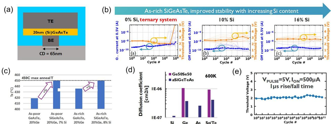
**Fig. 14** Ge-Te-As OTS selectors. **a** Device structure (65-nm plug). **b** Endurance of As-rich Ge-As-Te-Si OTS devices with different Si content. **c** Crystallization temperature, moving from Ge-Te-As to Ge-Te-As-Si system increases  $> 450$  °C. **d** Comparison of calculated element diffusion coefficient at 600 K for GeSe and Si-Ge-As-Te. **e** Endurance of  $10^{11}$  cycles achieved Ge-Te-As. Adapted with permission from [72]. Copyright 2019, IEEE
