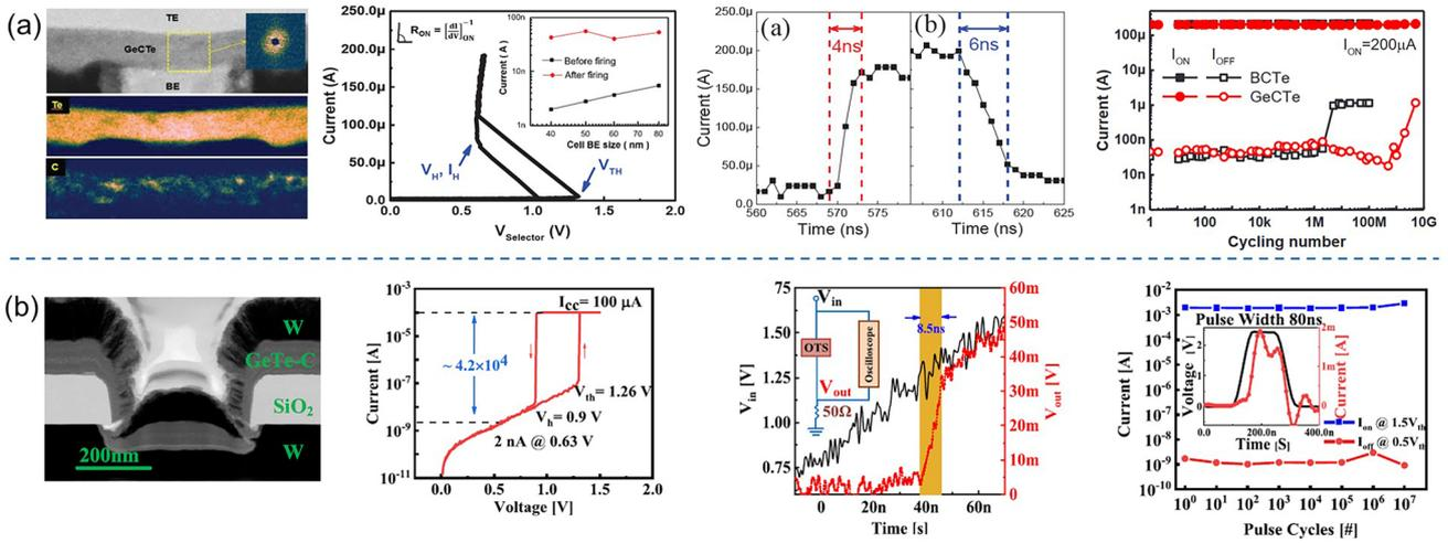
**Fig. 12** Ge–Te–C OTS selectors. **a** Device structure (30-nm plug), AC  $I$ – $V$  curves, switching speed, and endurance of Ge–Te–C OTS cells reported by Wu et al. [35]. **b** Device structure (250-nm BE), DC  $I$ – $V$  curves, on-switching speed, and endurance of Ge–Te–C OTS cells reported by Wang et al. Adapted with permission from [69], Copyright 2021, IEEE
