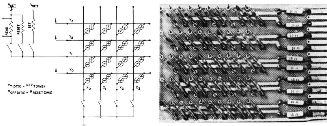
**Fig. 3** Schematic diagram and photograph of an OTS+OMS array. Adapted with permission from [17]. Copyright 1970, Elsevier
