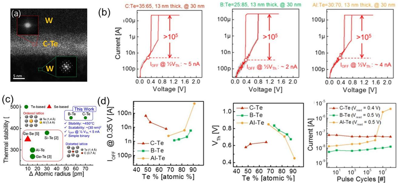
**Fig. 16** C–Te, B–Te, and Al–Te OTS selectors. **a** Device structure with 30–150 nm size. **b** DC *I*–*V* curves. **c** Relation between thermal stability and atomic radius difference. **d** *I*<sub>off</sub>, *V*<sub>th</sub> and endurance. Adapted with permission from [76]. Copyright 2018, IEEE
