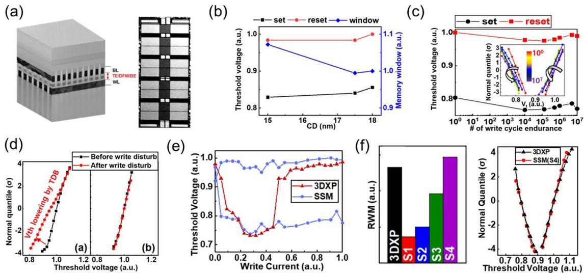
**Fig. 32** SSM prototype. **a** Structure of the SSM array. **b** Variations of  $V_{th}$  and the memory window with the device scaling down. **c** Endurance and the distribution of  $V_{th}$ . **d** Distribution of  $V_{th}$  before and after the driven thermal disturbance. **e**  $V_{th}$ – $I$  curves between 3D Xpoint and SSM. **f** Comparison of the margin window with 3D Xpoint [151]. Adapted with permission from [151]. Copyright 2022, IEEE
