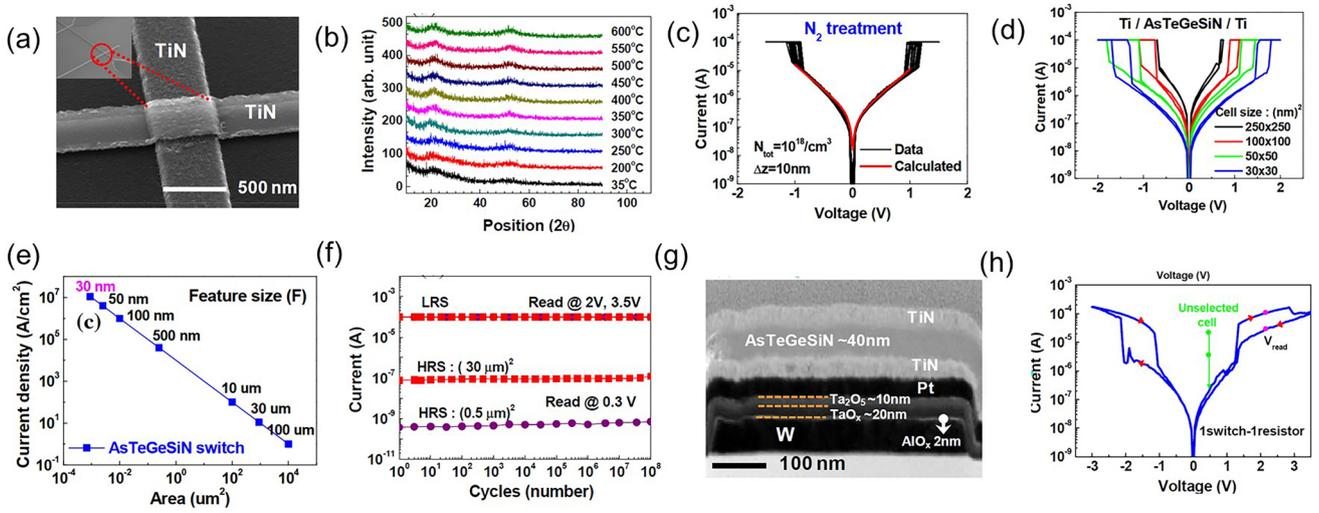
**Fig. 15** Ge–Te–As–Si–N OTS selector and 1S1R cell. **a** Device structure with 30 nm–100 μm size. **b** Thermal stability above 600 °C. **b** DC *I*–*V* curves. **c** DC *I*–*V* curves of the selector with varying sizes. **e** Scaling behavior. **f** Endurance. **g** 1S1R structure with Ta<sub>2</sub>O<sub>5</sub>/TaO<sub>x</sub> memory cell. **h** DC *I*–*V* curves of the 1S1R cell. Adapted with permission from [73]. Copyright 2012, IEEE
