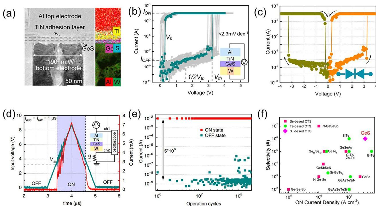
**Fig. 18** GeS OTS selectors. **a** Device structure with 190-nm plug. **b** DC  $I$ - $V$  curves. **c** DC bi-directional curves. **d** AC speed test. **e** Endurance  $> 10^8$ . **f** Comparison of selectivity and  $J_{on}$  of reported OTS devices [66]. Adapted with permission from [66]. Copyright 2020, Springer Nature
