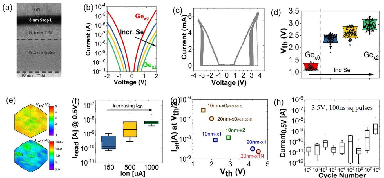
**Fig. 6** Ge–Se OTS selectors. **a** Device structure with 50-nm plug. **b** Leakage current. **c** AC  $I$ – $V$  curves. **d**  $V_{th}$  increase with higher Se content. **e**  $V_{th}$  and  $I_{off}$  distributions. **f**  $I_{on}$  vs. leakage current. **g**  $I_{off}$  comparison and **h** endurance. Adapted with permission from [38]. Copyright 2018, IEEE
