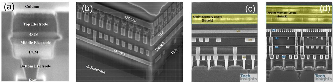
**Fig. 28** 1S1R structure in PCM. **a** Vertically integrated memory cell of 1S1R. **b** One layer of the PCM array fully integrated with CMOS [11, 12]. Adapted with permission from [11, 12]. Copyright 2009/2020, IEEE. **c** First-generation 2-deck 3D Xpoint array. **d** Second-generation 3D XPoint with 4-deck array [147]
