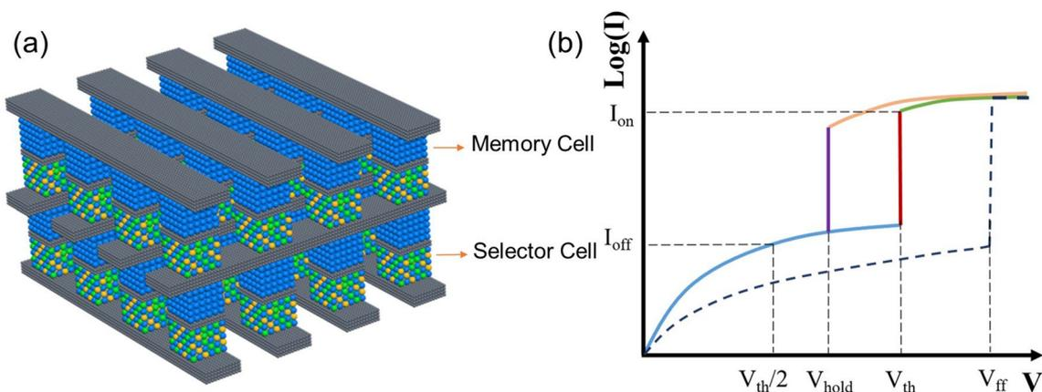
**Fig. 1** 3D Crosspoint architecture (a) and typical current–voltage ( $I$ - $V$ ) curve of the selector cell (b). A first fire voltage ( $V_{\text{ff}}$ ) is required to operate the selector cell. Then, a relative low voltage, called threshold voltage ( $V_{\text{th}}$ ), can turn on the cell, which would return to the off-state as the voltage decreases to the hold voltage ( $V_{\text{hold}}$ ).  $V_{\text{ff}} > V_{\text{th}} > V_{\text{hold}}$
