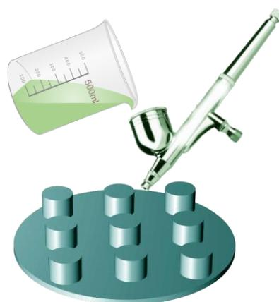
**Fig. S16** Schematic showing the fabrication process of various p-3DSE/LFP and p-3DSE/NCM811 cathodes by a simple spraying process
