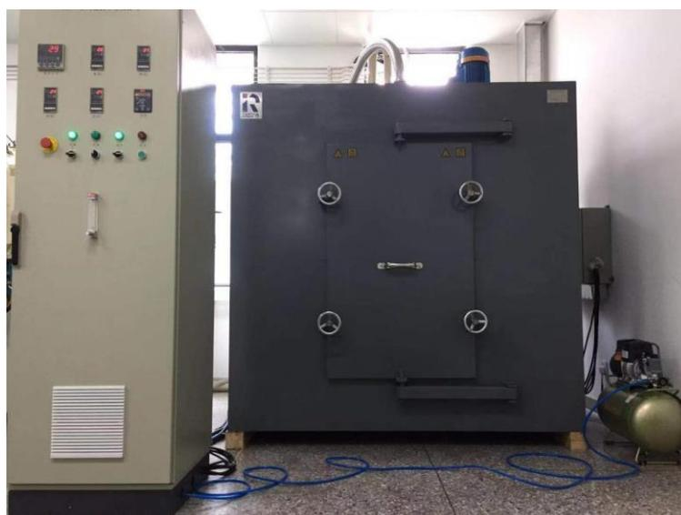
**Fig. S3** Carbonization furnace for high-temperature carbonization
