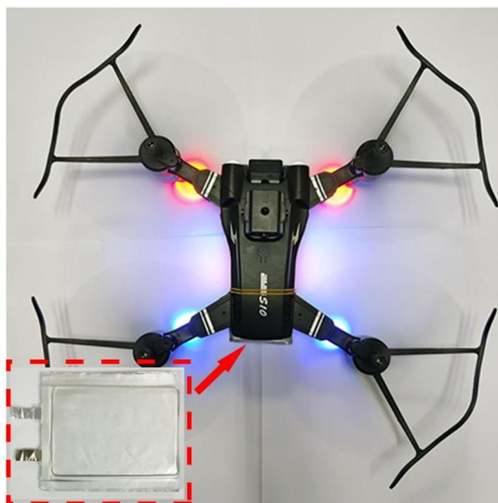
**Fig. 31** The drone powered by the prepared pouch full cell
