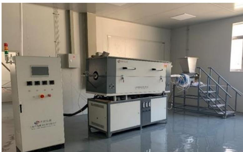
**Fig. S2** Rotary sealed box furnace for growing VG on the SiNDs/C
