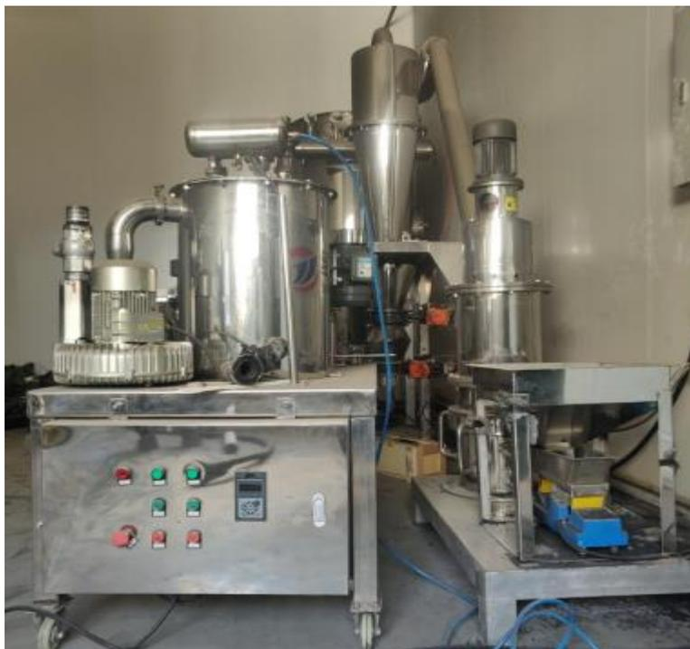
**Fig. S4** Airflow crusher for sample crushing
