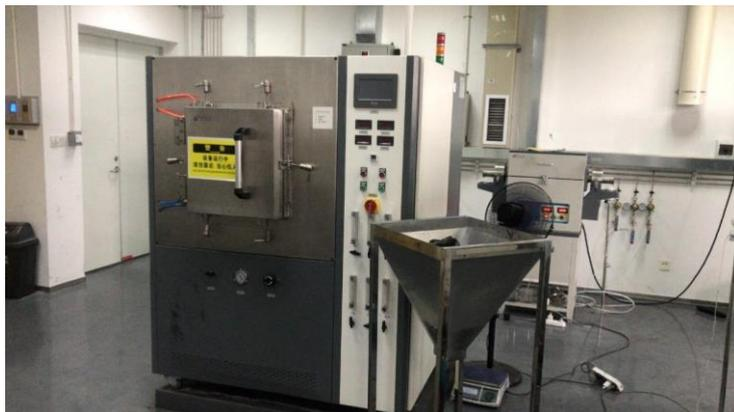
**Fig. S1** Static sealed box furnace for the production of the SiNDs/C
