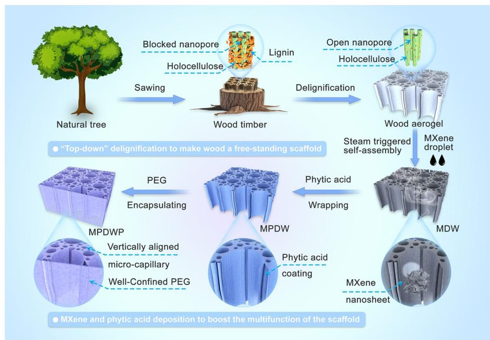
**Fig. 1** Schematic diagram of the preparation of composite phase change materials supported by phytic acid and MXene-decorated wood aerogel
