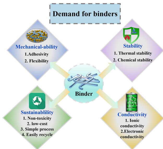
Fig. 3 Demand for cathode binders. Binders are crucial for cathode stability and performance, with PVDF being commonly used despite its drawbacks. Optimizing PVDF or finding alternatives is necessary. A qualified binder should meet cathode performance and sustainability goals. Providing with mechanical-ability, stability, sustainability, and conductivity
