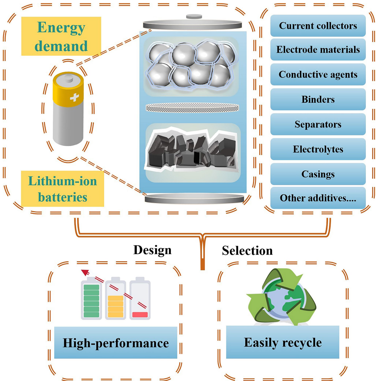
Fig. 1 Fossil fuel decline and pollution drive Li-ion battery innovation in energy density, stability, and sustainable recyclable component design. The depletion of fossil fuels and environmental pollution has driven a global trend toward renewable energy and energy efficiency. Lithium-ion batteries (LIBs) are key energy storage devices, and research focuses on enhancing their energy density and cycling stability. LFP and transition metal oxide cathodes are widely used, with LFP known for safety and stability. Transition metal oxide cathodes aim to increase energy density. Other battery components like conductive agents, binders, electrolytes, separators, current collectors, casings, and additives also influence battery performance. Their design and selection are crucial for energy density, power density, cycle life, safety, and cost. Batteries’ environmental and economic friendliness in recycling processes are also essential considerations
