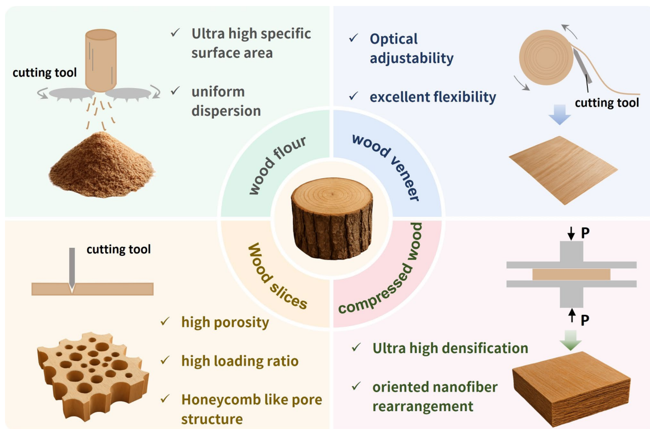
Fig. 3 Mechanical processing of wood into four forms—wood flour, veneer, slices, and compressed wood
