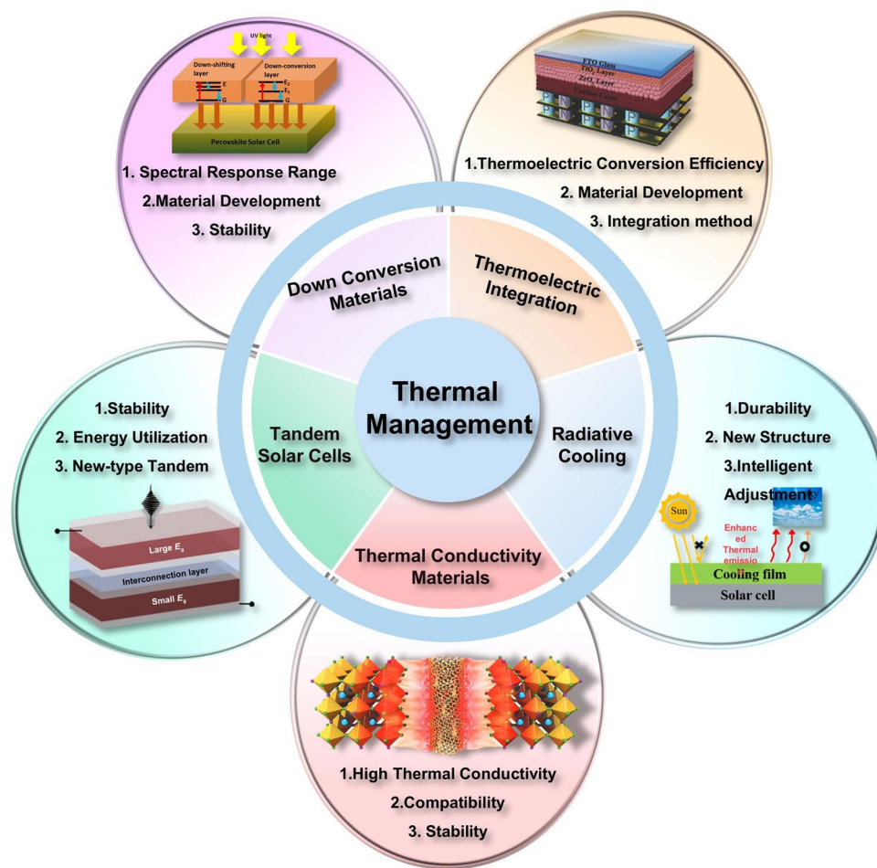
Fig. 9 Schematic diagram of thermal management strategies in PSCs, covering advanced thermal conductive materials [51], radiative cooling designs [84], thermoelectric integration [62], DC materials [87], and tandem architectures [126]
