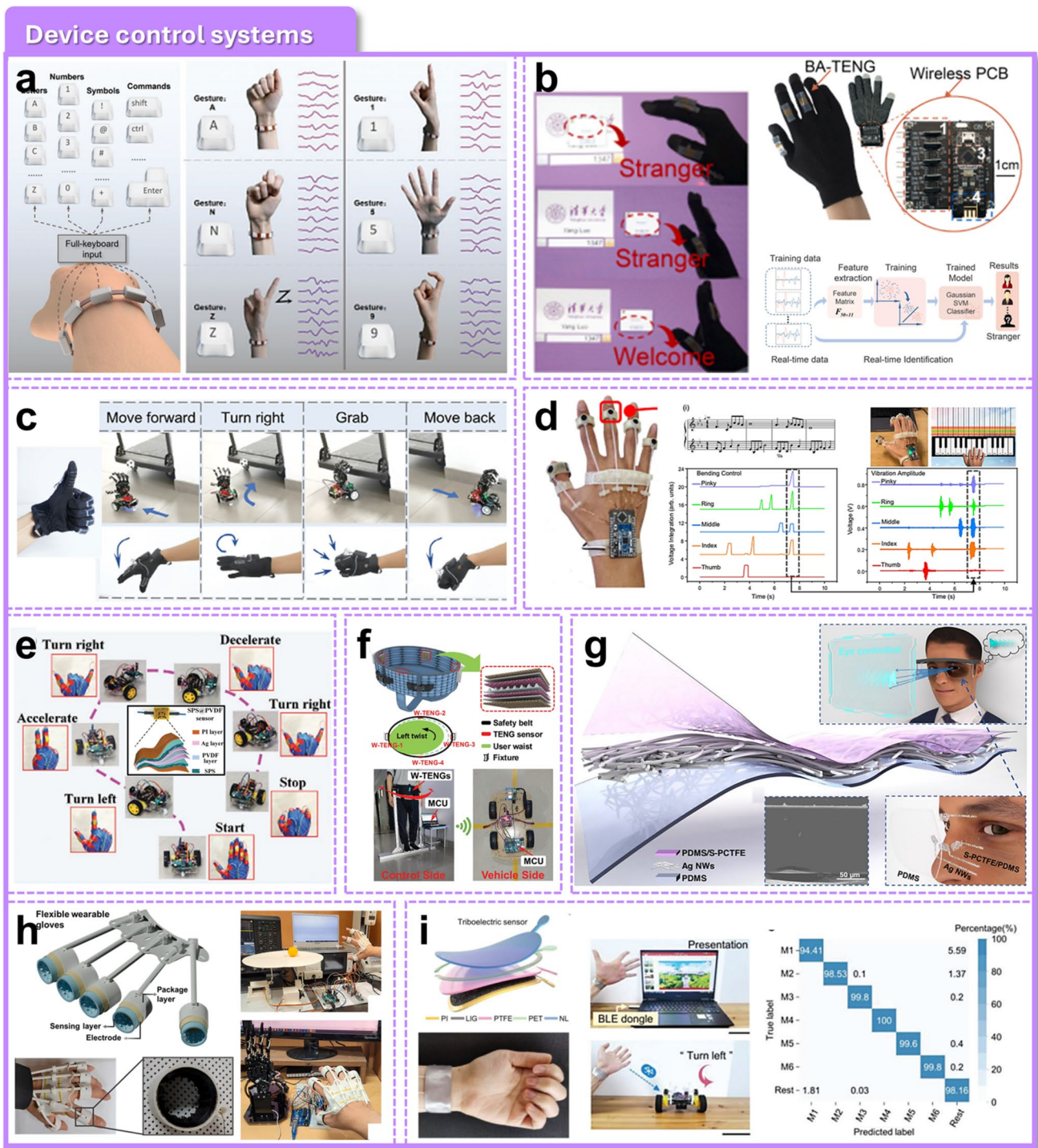
Fig. 11 Applications of device control. a Smart gesture recognition sensor for universal sign language. Reprinted with permission from Ref. [169]. © 2022 Wiley-VCH GmbH. b Smart glove based on triboelectric bending sensor. Reprinted with permission from Ref. [175]. © 2021 Elsevier Ltd. All rights reserved. c Playing virtual piano with multiple fingers. Reprinted with permission from Ref. [170]. © 2024 Linghong Ji et al., Advanced Science published by Wiley-VCH GmbH. d A self-powered intelligent shooting system for improving police shooting technology. Reprinted with permission from Ref. [172]. Copyright © 2022, Zhongda Sun et al. e Toy cars control by recognizing hand gesture. Reprinted with permission from Ref. [176]. © 2024 Wiley-VCH GmbH. f Smart belt based on TES to control the vehicle. Reprinted with permission from Ref. [163]. © 2021 Chengkuo Lee et al., Advanced Science published by Wiley-VCH GmbH. g TENG-based electrostatic interface for sensing eye tracking. Reprinted with permission from Ref. [161]. Copyright © 2023, Yuxiang Shi et al. h 3D-printed flexible wearable glove assembled with STTS. Reprinted with permission from Ref. [177]. © 2022 Elsevier Ltd. All rights reserved. i Triboelectric smart wristband for HMI. Reprinted with permission from Ref. [178]. © 2023 Hao Wu et al., Advanced Science published by Wiley-VCH GmbH
