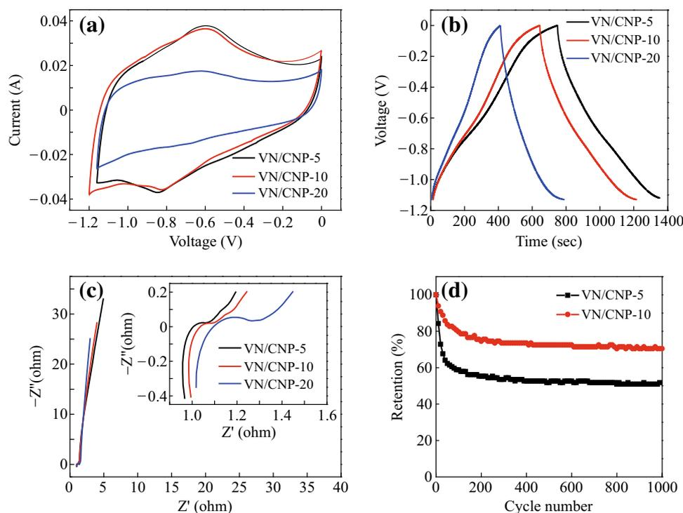
**Fig. 8** Comparisons of **a** CV, **b** galvanostatic charge–discharge curves, **c** complex-plane impedance plot, and **d** cycle life of VN/CNPs (scan rate =  $10 \text{ mV s}^{-1}$ , current density =  $1 \text{ A g}^{-1}$ ,  $2 \text{ M KOH}$  aqueous solution)
