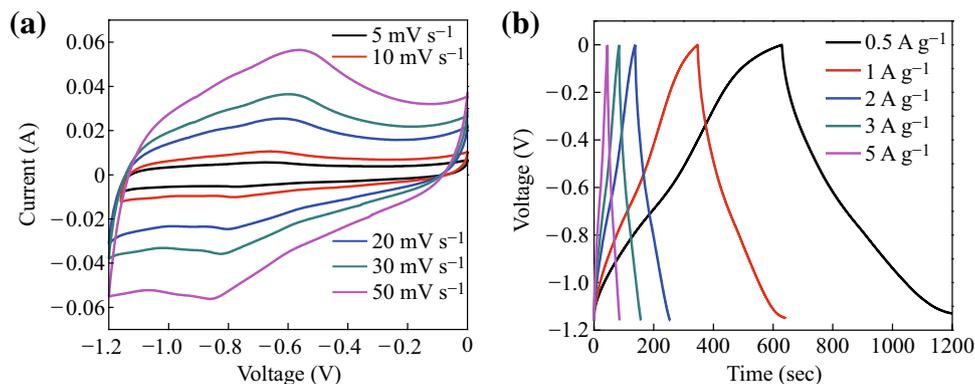
**Fig. 7** **a** CV at various scan rates (5–50  $\text{mV s}^{-1}$ ), and **b** galvanostatic charge–discharge curves at various currents (0.5–5  $\text{A g}^{-1}$ ) of VN/CNP-10
