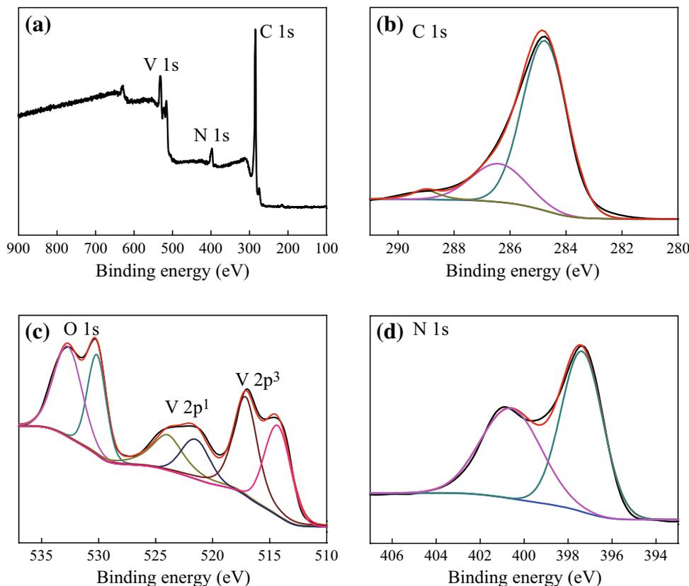
**Fig. 6** XPS spectra of **a** full scan, and curve fittings of **b** C 1s, **c** V 2p<sup>3</sup>, and **d** N 1s for VN/CNP-10
