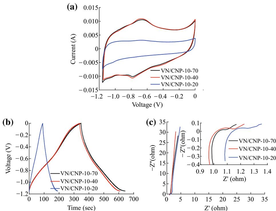
**Fig. 9** Comparisons of **a** CV, **b** galvanostatic charge–discharge, and **c** complex-plane impedance plots of VN/CNP-10-20, VN/CNP-10-40, and VN/CNP-10-70 (scan rate = 10 mV s<sup>-1</sup>, current density = 1 A g<sup>-1</sup>, 2 M KOH aqueous solution)
