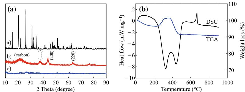
**Fig. 5** **a** The XRD patterns of *a*  $V_2O_5$  powder, *b* VN/CNP-10, and *c*  $V_2O_5$  xerogel. **b** The TGA and DSC analysis of VN/CNP-10
