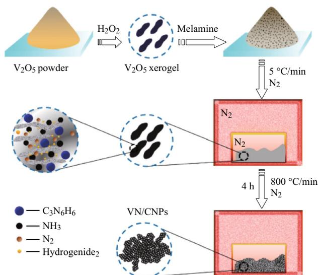
**Scheme 1** Schematic illustration for the preparation of VN/CNPs
