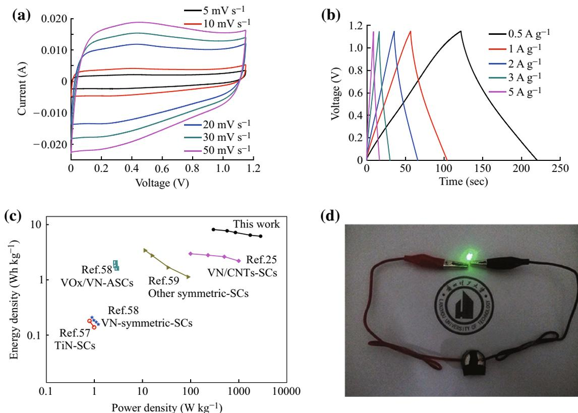
**Fig. 10** **a** CV, and **b** galvanostatic charge–discharge curves of the hybrid supercapacitor. **c** Ragone plots of the VN/CNP symmetric supercapacitor, and the values reported for other SC devices for comparison [25, 57–59]. **d** Green LED was powered by the tandem VN/CNP-SSCs. (scan rate =  $10 \text{ mV s}^{-1}$ , current density =  $1 \text{ A g}^{-1}$ ,  $2 \text{ M KOH}$  aqueous solution)
