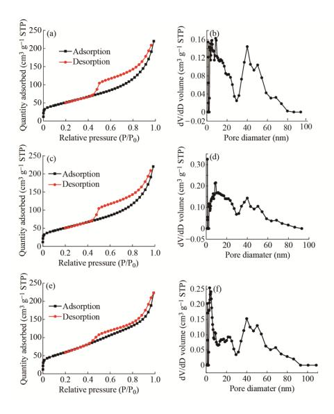
**Figure S1** Nitrogen adsorption-desorption isotherms, and pore size distribution of (**a** and **b**) VN/CNPs-10-20, (**c** and **d**) VN/CNPs-10-40, and (**e** and **f**) VN/CNPs-10-70
