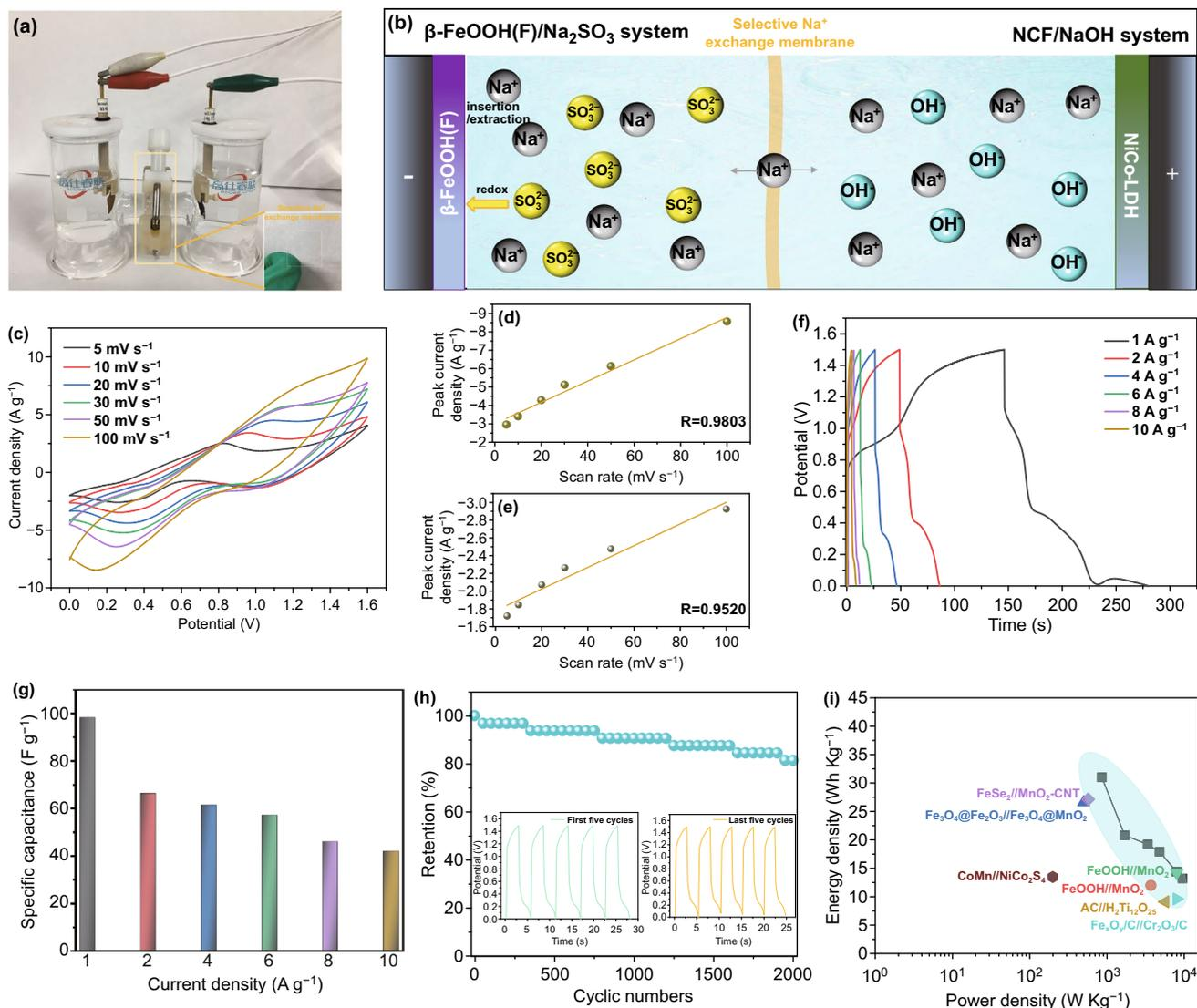
**Fig. 5** **a** Optical image and **b** scheme of dual electrolyte asymmetric supercapacitor (DESC). **c–i** Electrochemical performances: **c** CVs, **d** peak current density versus scan rate and **e** scan rate<sup>-1/2</sup>, **f** GCDs, **g** rate capacity, **h** cycling stability, inset the first and last five cycles, **i** Ragone plot
