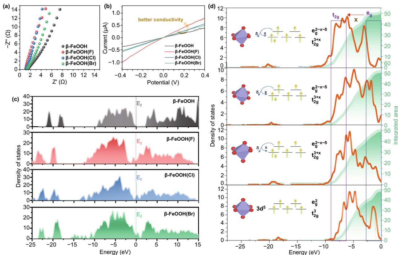
**Fig. 3** **a** EIS, **b**  $I$ - $V$ , **c** DOS curves, and **d** PDOS of Fe 3d valence band orbitals of  $\beta$ -FeOOH and  $\beta$ -FeOOH(X)s
