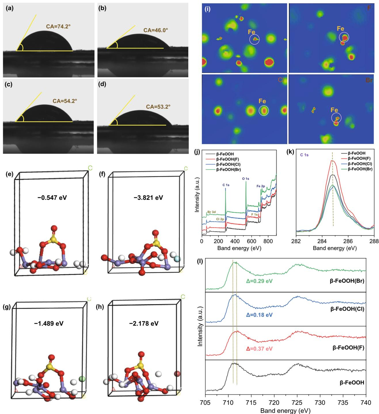
**Fig. 4** a–d Contact angles, e–h adsorption energies for  $\text{SO}_3^{2-}$ , i charge density differential diagram, j–l XPS of  $\beta\text{-FeOOH}$  and  $\beta\text{-FeOOH(X)}$ s
