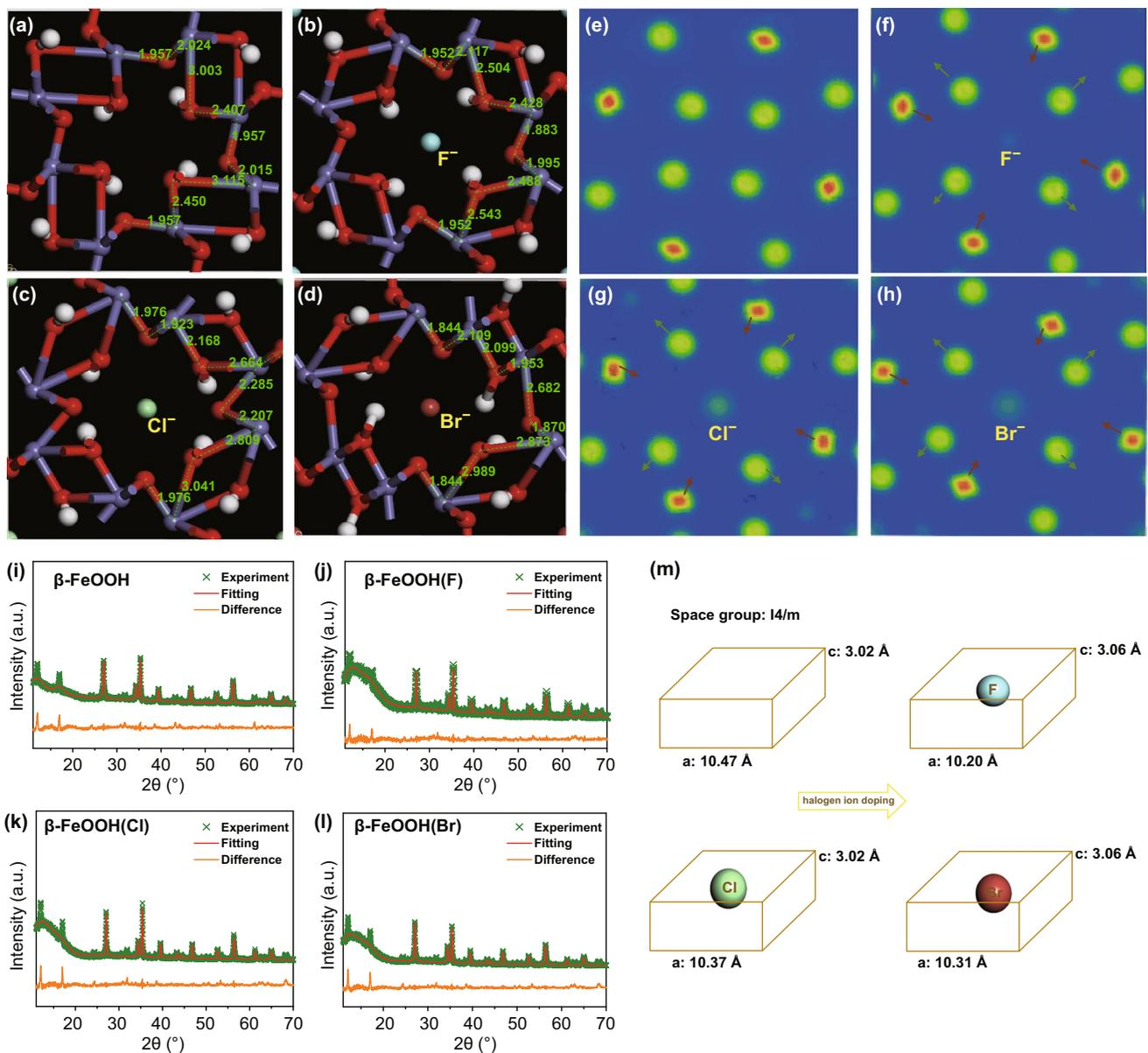
**Fig. 1** a–d DFT calculation, e–h the corresponding charge density differential diagram, and i–l Rietveld XRD patterns of  $\beta$ -FeOOH and  $\beta$ -FeOOH(X)s. m Corresponding schematic illustration of the contraction of  $\beta$ -FeOOH cell after doping halogen ions
