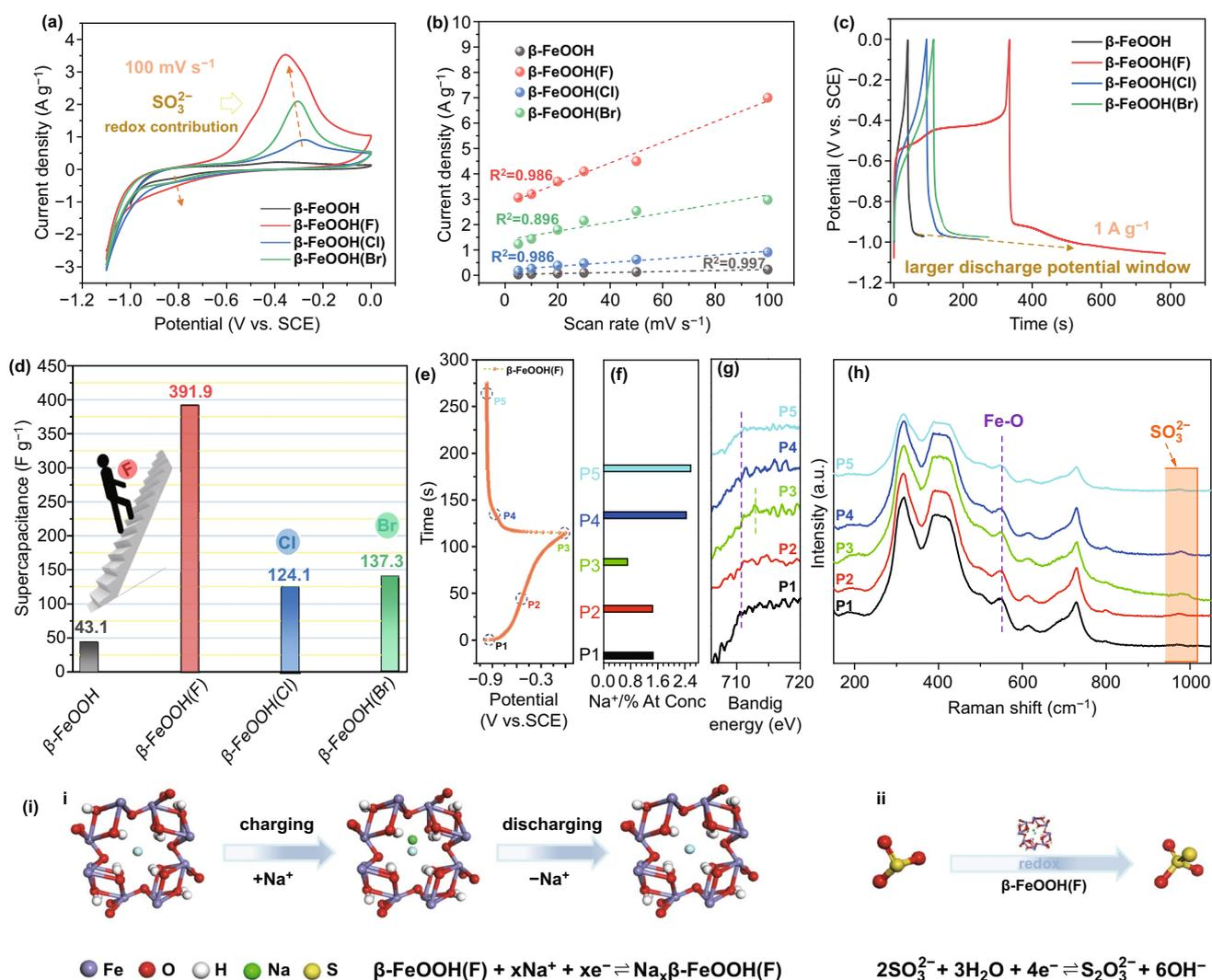
**Fig. 2** Electrochemical performances of  $\beta$ -FeOOH and  $\beta$ -FeOOH(X)s. **a** CVs, **b** plots of peak current density versus scan rate, **c** GCDs, **d** comparison of specific capacity, **e–h** ex situ XPS and Raman of  $\beta$ -FeOOH(F) under different charge/discharge potentials, and **i** scheme of energy storage mechanism of  $\beta$ -FeOOH(F)
