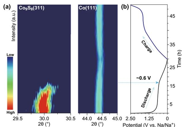
**Fig. 5** *Operando* XRD patterns collected at various states of the initial discharge/charge process of a  $\text{Co}_9\text{S}_8@\text{NC-9}$ /sodium electrochemical cell. Contour plots of the diffraction peak evolution of  $\text{Co}_9\text{S}_8$  (311) and Co (111) planes. The corresponding galvanostatic discharge–charge profiles at a current density of  $20 \text{ mA g}^{-1}$  from the open circuit potential to 0.01 V
