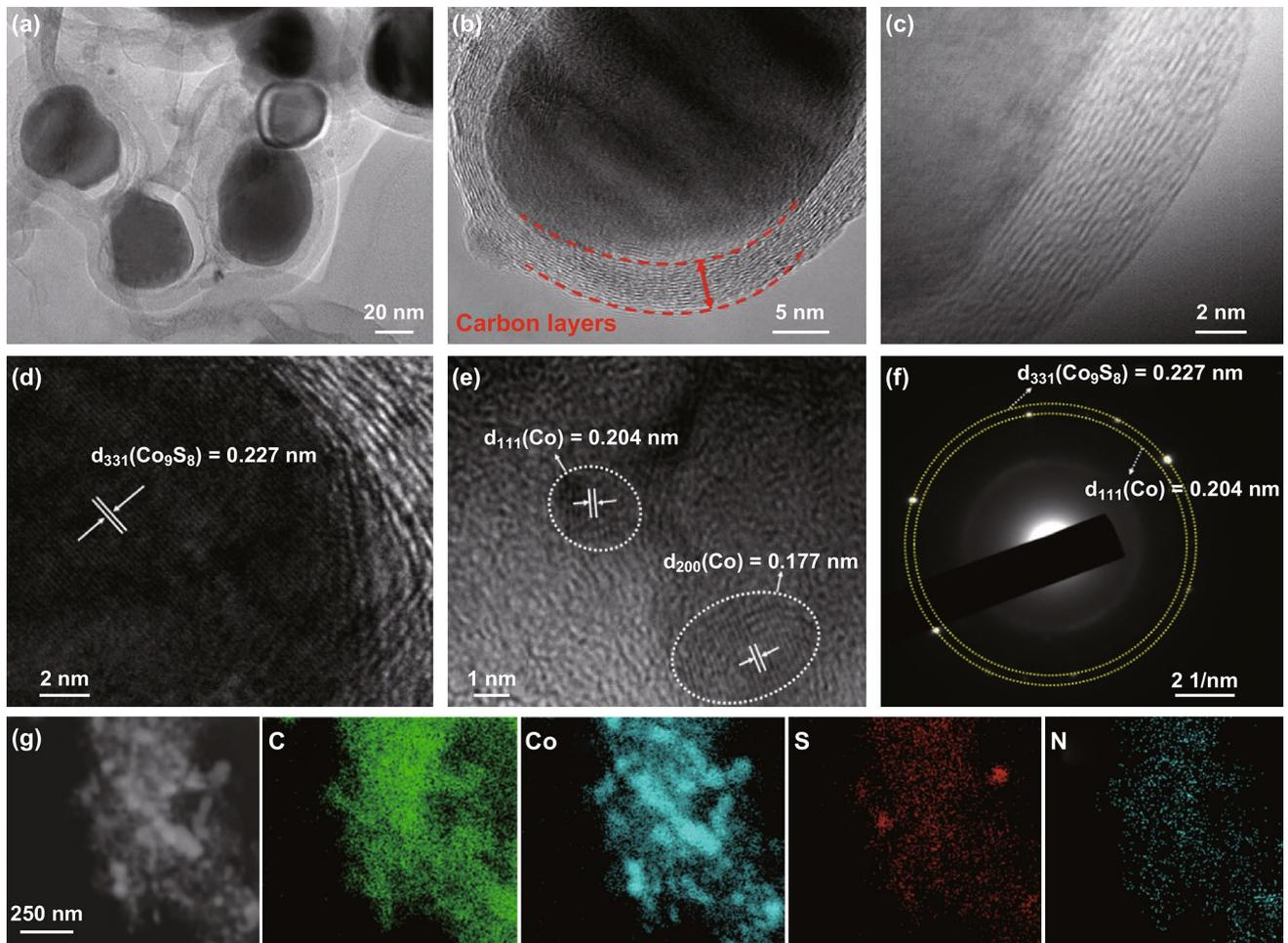
**Fig. 2** Morphology and structure of the as-prepared  $\text{Co}_9\text{S}_8@\text{NC-9}$ . **a–c** TEM images with different magnifications. **d, e** HRTEM images presenting the lattice fringes. **f** SAED pattern. **g** Elemental mapping images showing the distribution of C, Co, S, and N elements
