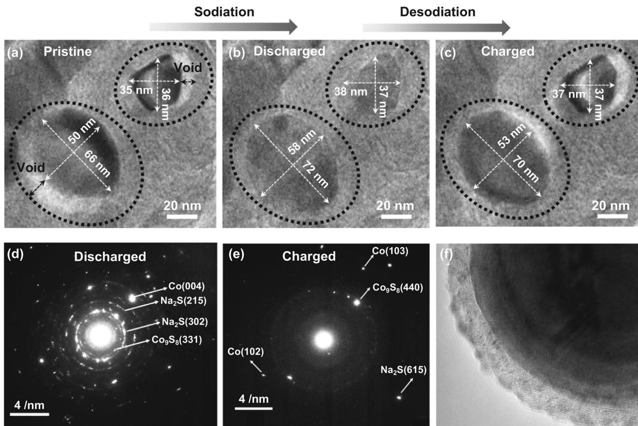
**Fig. 4** a–c *In situ* TEM investigation of structural changes of the  $\text{Co}_9\text{S}_8@\text{NC}$  electrode during varied sodiation depths. SAED patterns the  $\text{Co}_9\text{S}_8@\text{NC}$  electrode at **d** sodiated to 0.01 V and **e** desodiated to 2.5 V illustrating the compositional changes. **f** HRTEM images of  $\text{Co}_9\text{S}_8@\text{NC}$  electrode after long-term cycling after 400 cycles
