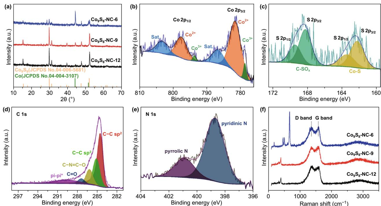
**Fig. 1** **a** XRD pattern of the  $\text{Co}_9\text{S}_8@\text{NC}$  composites and the standard XRD patterns of  $\text{Co}$  (JCPDS No. 04-004-3107) and  $\text{Co}_9\text{S}_8$  (JCPDS No. 04-006-5681). **b–e** High-resolution XPS spectra of  $\text{Co}_9\text{S}_8@\text{NC-9}$ . **f** Raman spectra of the  $\text{Co}_9\text{S}_8@\text{NC}$
