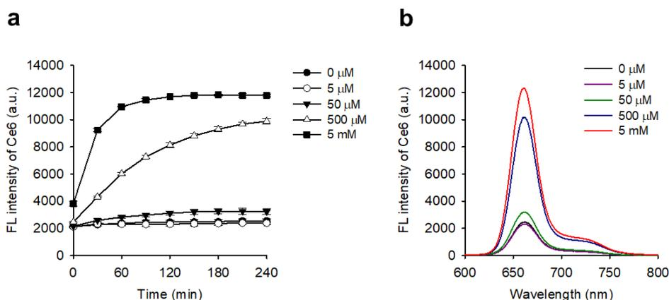
**Fig. S2** (a) Recovery in NIR fluorescence of CFN-gel over time after addition of various concentrations of reducing agent DTT. (b) Fluorescence spectra of CFN-gel at 2 μM of Ce6 equivalent after incubation in 0-5 mM DTT solution for 4 h ( $\lambda_{ex} = 400$  nm)
