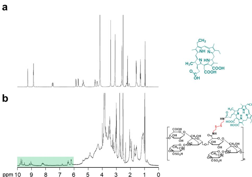
**Fig. S1** <sup>1</sup>H-NMR spectra of (a) Ce6 and (b) CFN-gel dissolved in d<sub>6</sub>-DMSO/D<sub>2</sub>O. The degree of conjugation of Ce6 per a fucoidan molecule was calculated by comparing the peak area at the two intense unresolved peaks at 0.96 and 1.12 ppm (corresponding to the methyl groups of fucose units) and 6.0–7.0 ppm (corresponding to -CH=CH<sub>2</sub> of Ce6) of <sup>1</sup>H-NMR spectrum [S1-S3]
