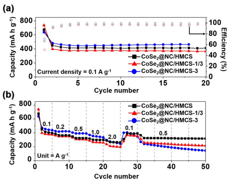
**Fig. S17** Electrochemical properties of CoSe<sub>2</sub>@NC/HMCS composites with different amount of Co-nitrate: **a** cycle performances at a current density of 0.1 A g<sup>-1</sup>, and **b** rate performances at various current densities
