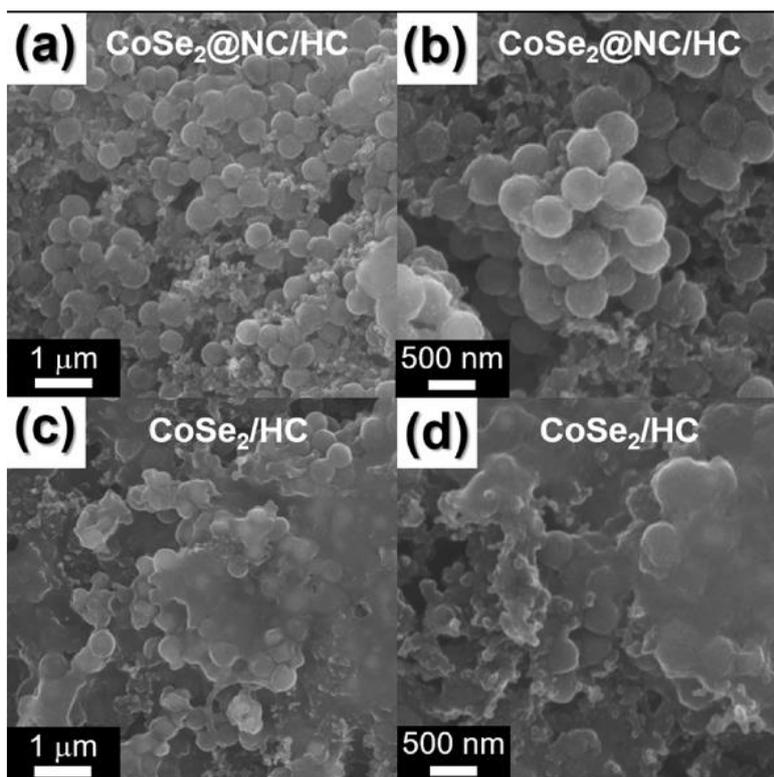
**Fig. S11** Morphologies of **a, b** CoSe<sub>2</sub>@NC/HMCS and **c, d** CoSe<sub>2</sub>/HMCS composites after 100 cycles
