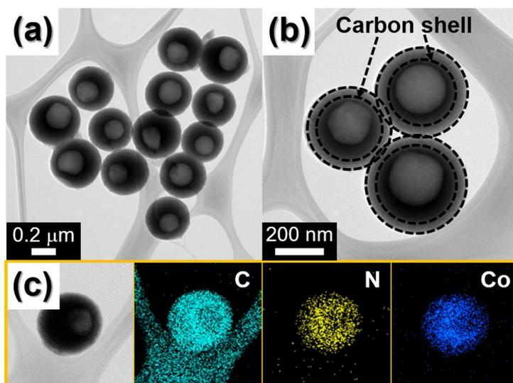
**Fig. S2** Morphologies and elemental mapping images of ZIF-67/HMCS composite prepared under vacuum state: **a, b** TEM images and **c** elemental mapping images
