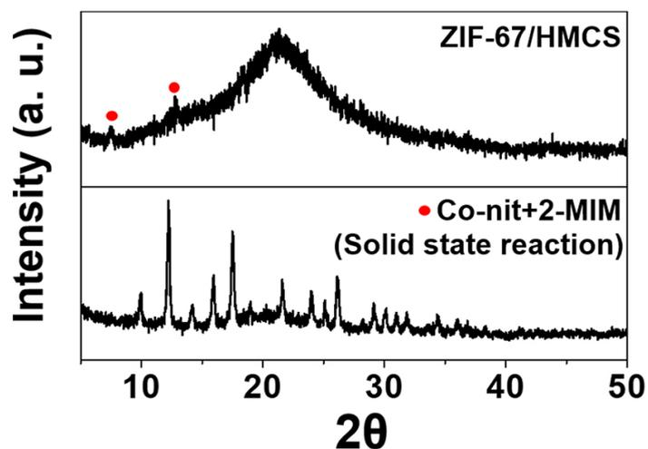
**Fig. S3** XRD patterns of ZIF-67/HMCS composite and powders formed by solid-state reaction of cobalt salt and 2-methylimidazole at 180 °C
