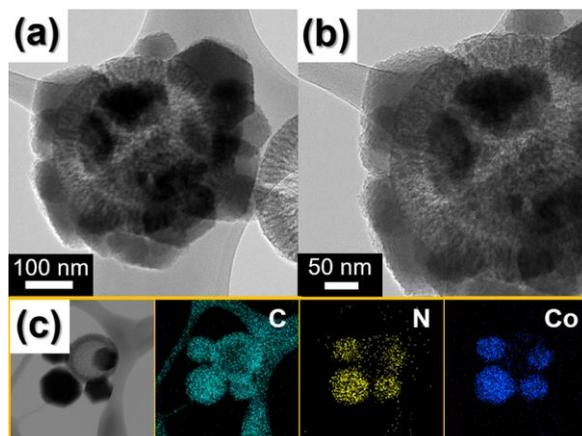
**Fig. S6** Morphologies and elemental mapping images of ZIF-67/HMCS composite prepared under non-vacuum state: **a, b** TEM images and **c** elemental mapping images
