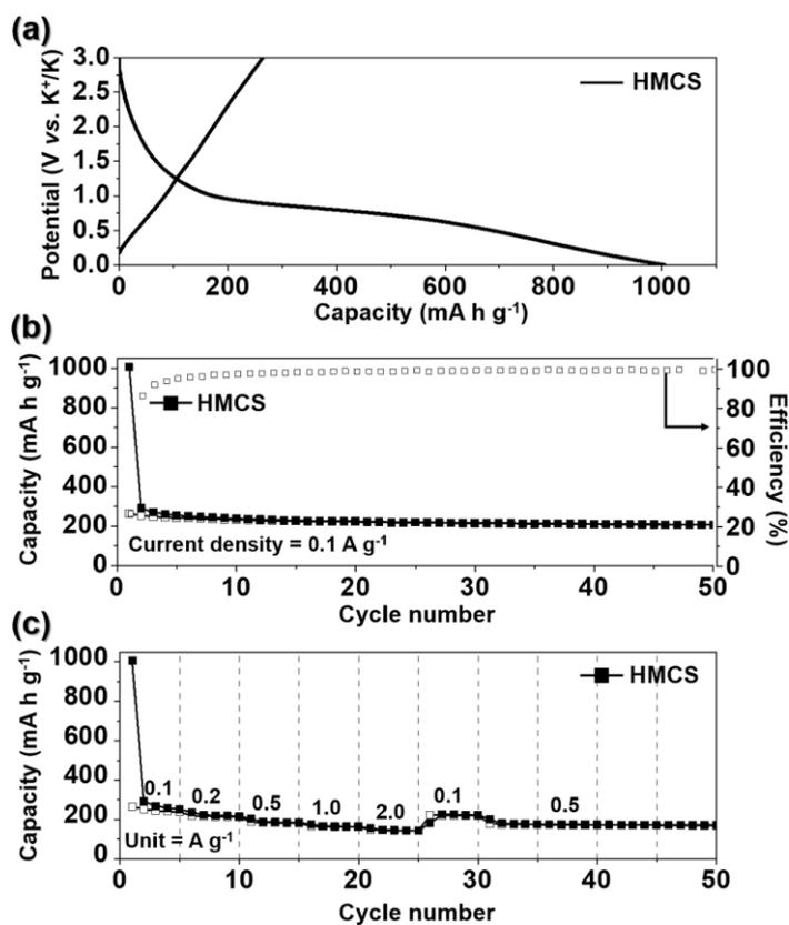
**Fig. S12** Electrochemical properties of HMCS: **a** initial galvanostatic charge-discharge curves, **b** cycle performance at a current density of 0.1 A g<sup>-1</sup>, and **c** rate performance at various current densities
