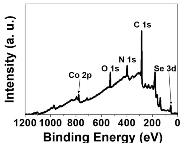
Fig. S8 XPS survey scan for CoSe<sub>2</sub>@NC/HMCS composite
