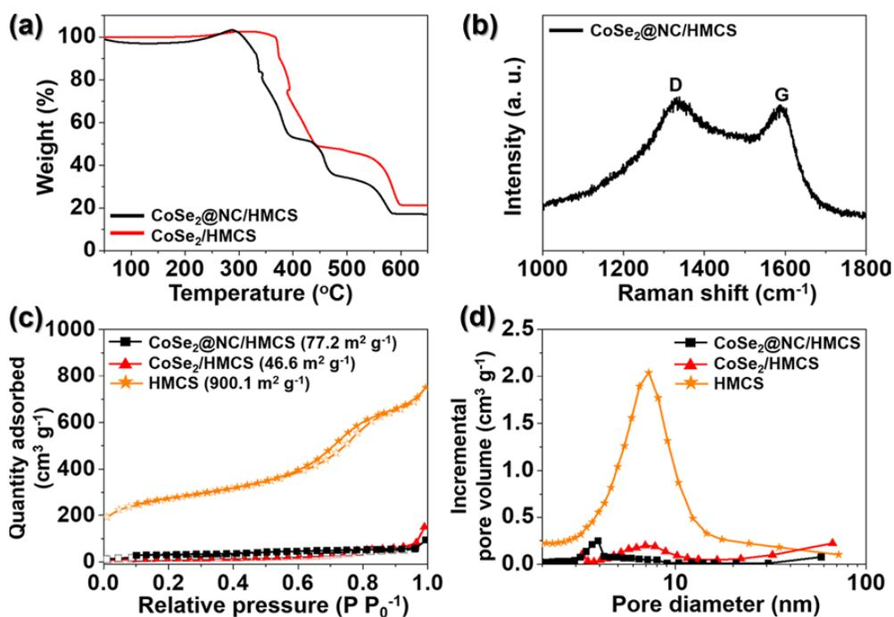
Fig. S9 a TG curves, b Raman spectra, c N<sub>2</sub> gas adsorption and desorption isotherms, and d BJH pore size distributions of HMCS, CoSe<sub>2</sub>@NC/HMCS, and CoSe<sub>2</sub>/HMCS composites
