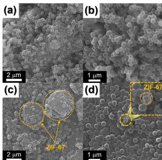
**Fig. S5** Morphologies of Co-nitrate/HMCS and ZIF-67/HMCS composites synthesized under non-vacuum state: **a, b** SEM images of Co-nitrate/HMCS and **c, d** SEM images of ZIF-67/HMCS
