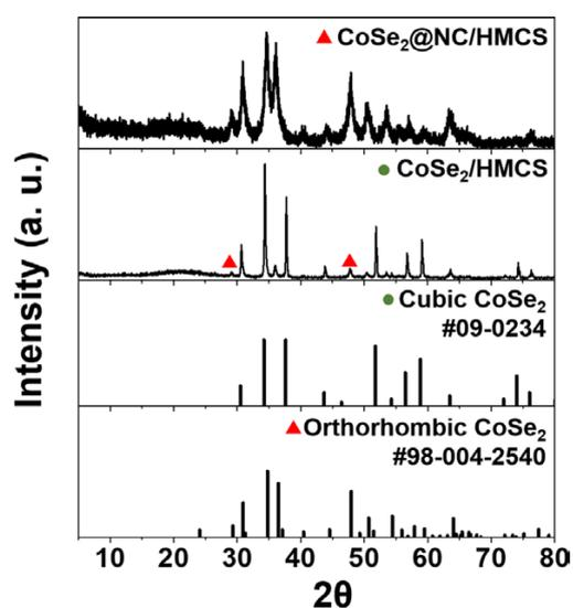
**Fig. S7** XRD patterns of of CoSe<sub>2</sub>@NC/HMCS and CoSe<sub>2</sub>/HMCS composites
