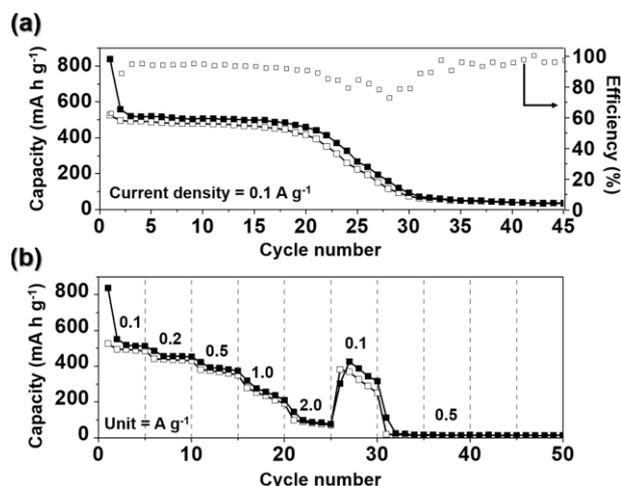
**Fig. S15** Electrochemical properties of CoSe<sub>2</sub>@NC/HMCS composite prepared under non-vacuum state: **a** cycle performance at a current density of 0.1 A g<sup>-1</sup> and **b** rate performance at various current densities
