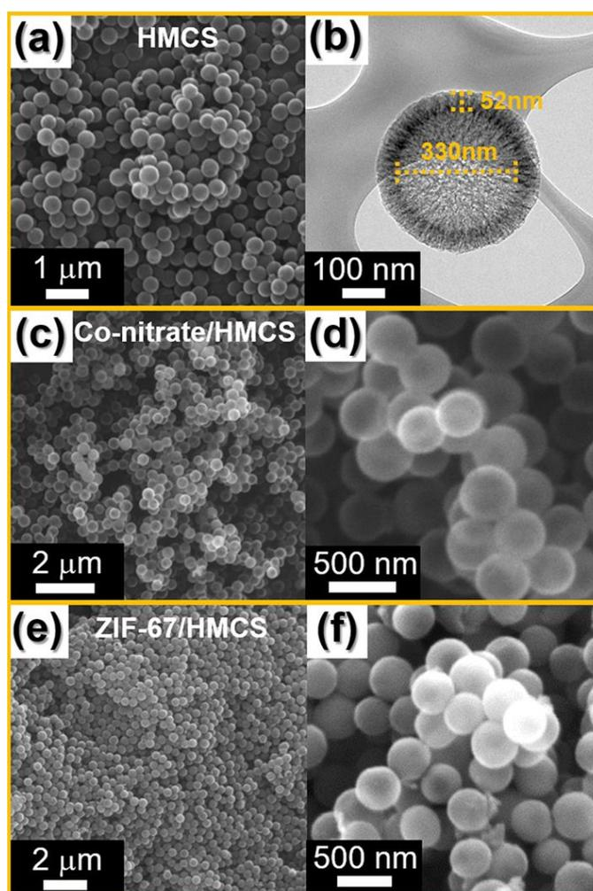
**Fig. S1** Morphologies of HMCS, Co-nitrate/HMCS, and ZIF-67/HMCS prepared under vacuum state : **a, b** SEM image and TEM image of HMCS, **c, d** SEM images of Co-nitrate/HMCS, and **e, f** SEM images of ZIF 67/HMCS
