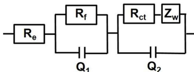
Fig. S10 Randle-type equivalent circuit model used for EIS fitting
