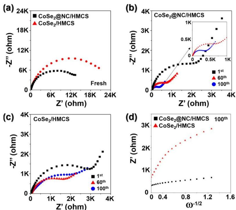
**Fig. S18** Nyquist plots of **a** fresh cells, **b** after the 1<sup>st</sup>, 60<sup>th</sup>, and 100<sup>th</sup> cycle of CoSe<sub>2</sub>@NC/HMCS composite, **c** after the 1<sup>st</sup>, 60<sup>th</sup>, and 100<sup>th</sup> cycle of CoSe<sub>2</sub>/HMCS composite, and **d** the relationship between the phase angle ( $\omega^{-1/2}$ ) and impedance ( $Z'$ ) of the two electrodes at the 100<sup>th</sup> cycle
