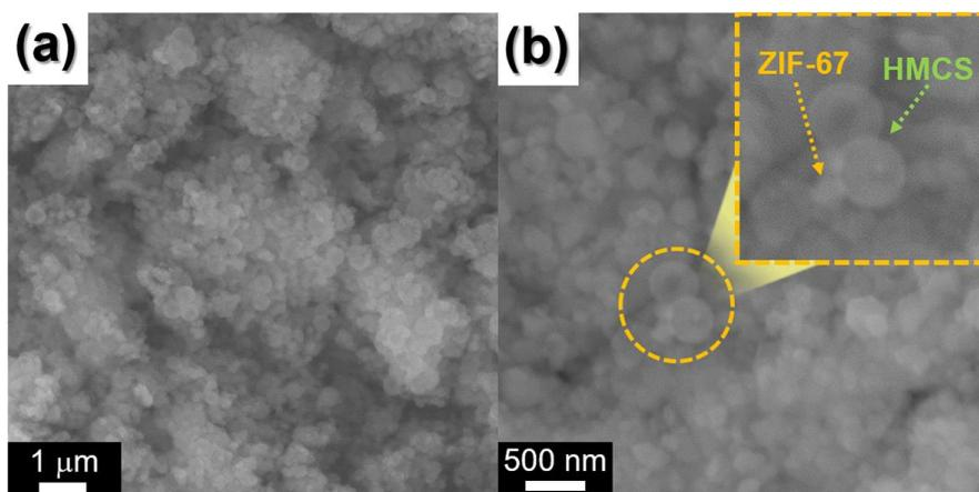
**Fig. S4** Morphologies of ZIF-67/HMCS composite prepared by liquid-phase process: **a, b** SEM images
