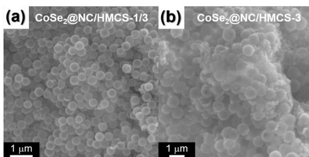
**Fig. S16** Morphologies of CoSe<sub>2</sub>@NC/HMCS-1/3 and CoSe<sub>2</sub>@NC/HMCS-3 composites: **a**, **b** SEM images
