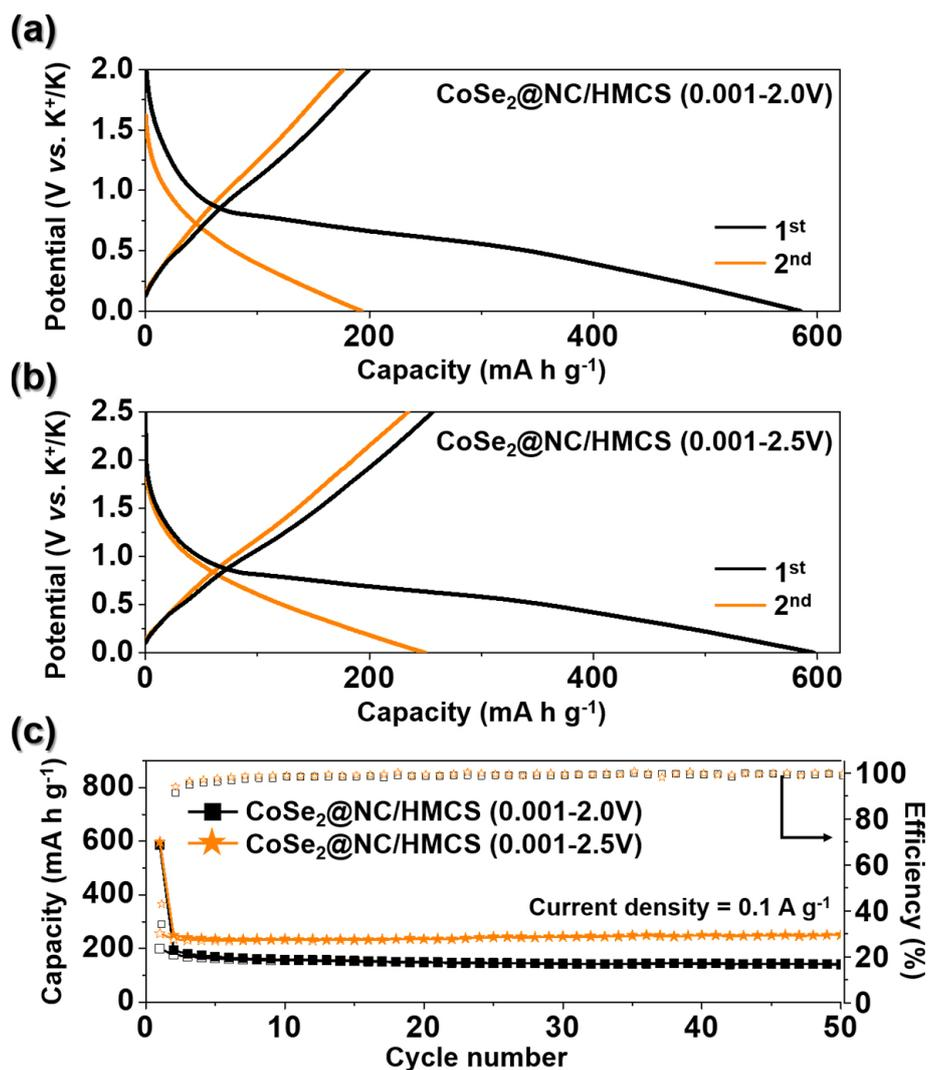
**Fig. S13** Electrochemical properties of  $\text{CoSe}_2@NC/HMCS$  composite in the range of 0.001-2.0 and 0.001-2.5 V: **a, b** the first and second galvanostatic charge-discharge curves, **b** cycle performances at a current density of  $0.1 \text{ A g}^{-1}$
