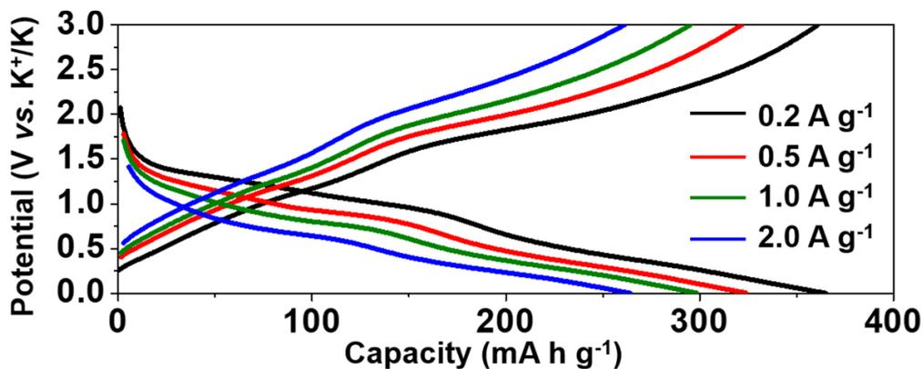
**Fig. S14** Galvanostatic charge-discharge curves of  $\text{CoSe}_2@NC/HMCS$  composite at various current densities
