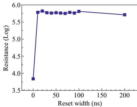
**Fig. 3**  $T$ - $R$  curve of the RESET operation for the 1T1R memory cell
