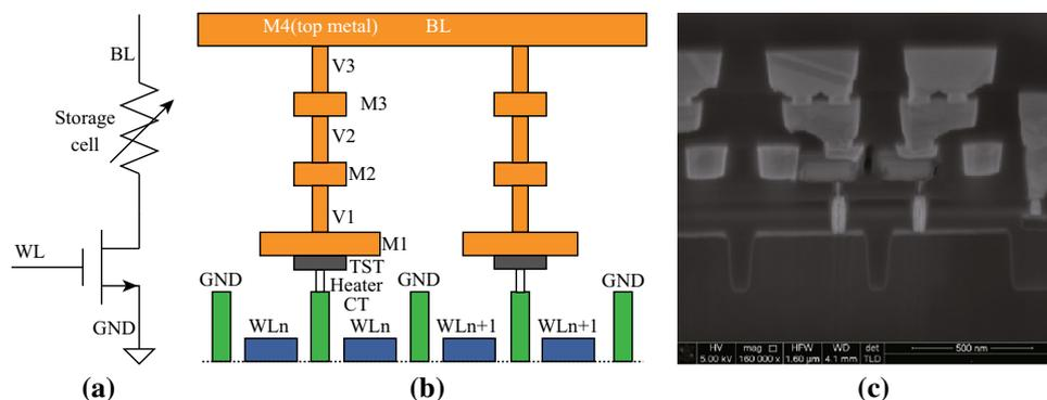
**Fig. 1** a Schematic of the 1T1R structure memory cell. b Schematic cross section of the 1T1R structure. c SEM image of a detail of the array along the WL direction
