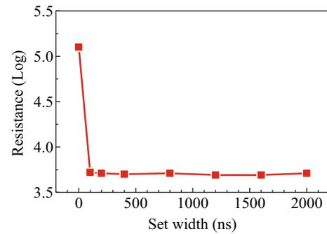
**Fig. 5**  $T$ - $R$  curve the SET operation for the 1T1R memory cell
