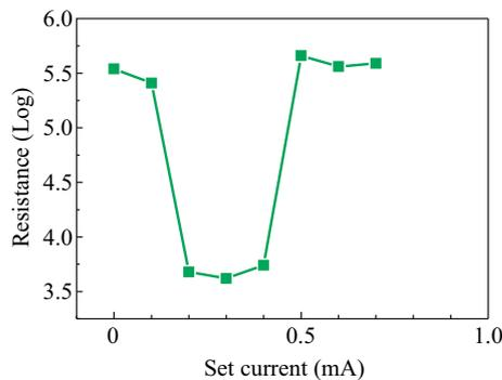
**Fig. 4**  $I$ - $R$  curve of the SET operation for the 1T1R memory cell
