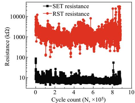
**Fig. 7** Reset/set endurance value for the memory cell
