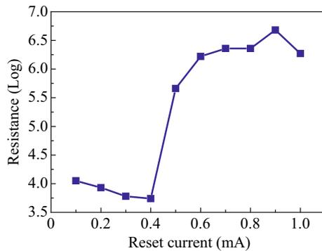
**Fig. 2**  $I$ - $R$  curve of the RESET operation for the 1T1R memory cell
