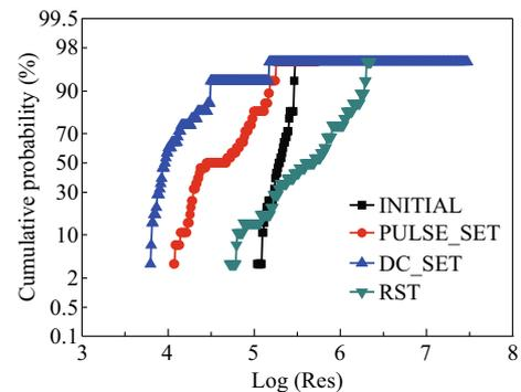
**Fig. 6** Resistance value distribution for the experimental chip
