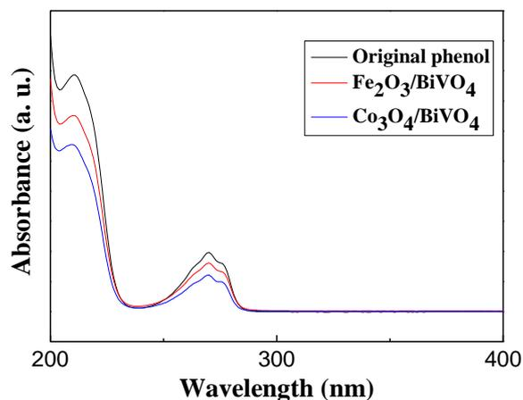
**Fig. S12** The adsorption behavior of phenol on  $\text{Fe}_2\text{O}_3/\text{BiVO}_4$  and  $\text{Co}_3\text{O}_4/\text{BiVO}_4$
