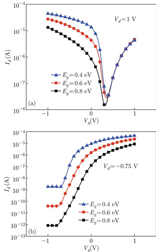
Fig. 5 Calculated transfer characteristics of the CNT-FETs with different SWNT band gaps for  $V_d = 1$  V (a) and  $V_d = -0.75$  V (b). The blue, red, and black curves are for  $E_g = 0.4, 0.6$  and  $0.8$  eV, respectively.
