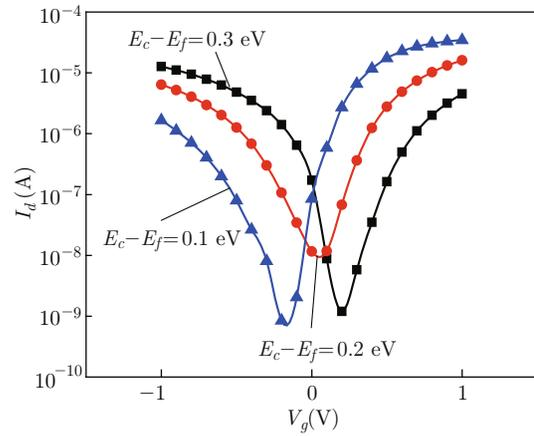
Fig. 3 Calculated transfer characteristics of the CNTFETs with different Si doping level at  $V_d = 0.75$  V. The black, red and blue curves are for  $E_c - E_f = 0.3, 0.2$  and  $0.1$  eV, respectively. The band gap of the SWNT is 0.6 eV.
