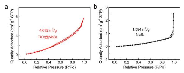
Fig. S4 BET measurements: nitrogen adsorption-desorption isotherm curves: a TiO<sub>2</sub>@Ni<sub>3</sub>S<sub>2</sub> nanowire arrays and b Ni<sub>3</sub>S<sub>2</sub> arrays
