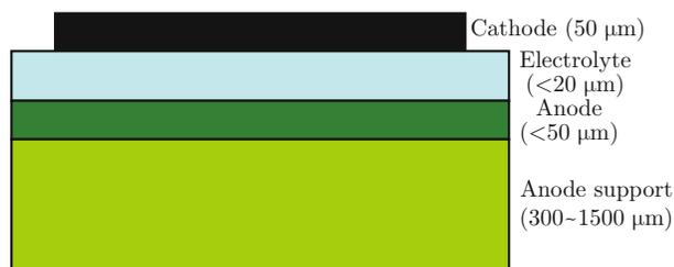
Fig. 1 Structure of typical anode-supported SOFC.
