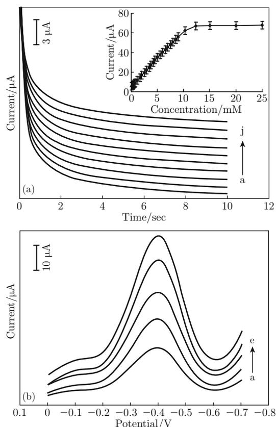
Fig. 6 (a) Amperometric response of MWCNT-NR-GO<sub>x</sub>-HRP-Nf biocomposite electrode (a-j) for the successive addition of 0.1 M H<sub>2</sub>O<sub>2</sub> in 0.1 M PB (pH=7.4); Inset shows the linear calibration plot. (b) Differential pulse voltammograms of nanobiocomposite biosensor (a-e) at successive addition 1.0 M H<sub>2</sub>O<sub>2</sub>.
