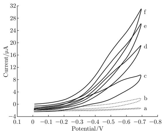
Fig. 3 Cyclic voltammograms of bare GCE (a) without  $\text{H}_2\text{O}_2$  (b) with  $3.0 \mu\text{M}$   $\text{H}_2\text{O}_2$  and (c, d, e, f) MWNTs/NR/GOx/HRP/Nf modified GCE in  $0.1 \text{ M}$   $7.4$  PBS containing  $0$ ,  $1.0$ ,  $2.0$  and  $3.0 \text{ M}$   $\text{H}_2\text{O}_2$  at  $0.20 \text{ V/s}$ .
