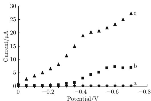
Fig. 5 Hydrodynamic voltammograms for 3.0 M H<sub>2</sub>O<sub>2</sub> in 0.1 M phosphate buffer solution (pH=7.4) at (a) unmodified (b) MWCNT-GO<sub>x</sub>-HRP-Nf modified and (c) MWCNT-NR-GO<sub>x</sub>-HRP-Nf modified GC electrodes.
