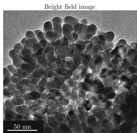
Fig. 2 TEM bright field image of as-synthesized nanoparticles.
