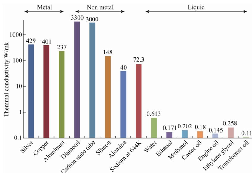
FIG. 2. Comparison of thermal conductivity for different materials.
