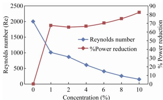
FIG. 3. Comparison of Reynolds number and percent power reduction for different concentration of Al<sub>2</sub>O<sub>3</sub> nanofluid.
