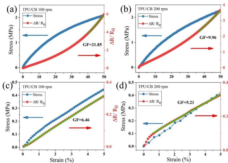
**Fig. S5** The normalized change of **a** RS-100 and **b** RS-200 under 0-50% strain and under **c, d** 0-5% in tensile stress and electrical resistance ( $\Delta R/R_0$ ) vs. strain.
