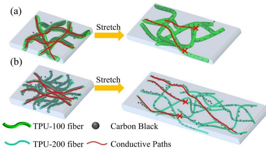
**Fig. S6** Schematics of the morphology change of stretched (c) RS-100 and (d) RS-200 strain sensor
