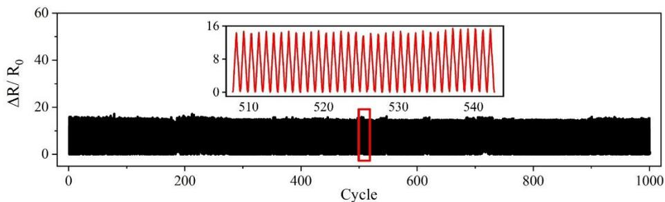
**Fig. S4** 1000 stretching-releasing cycles toward the strain variation from 0 to 50%
