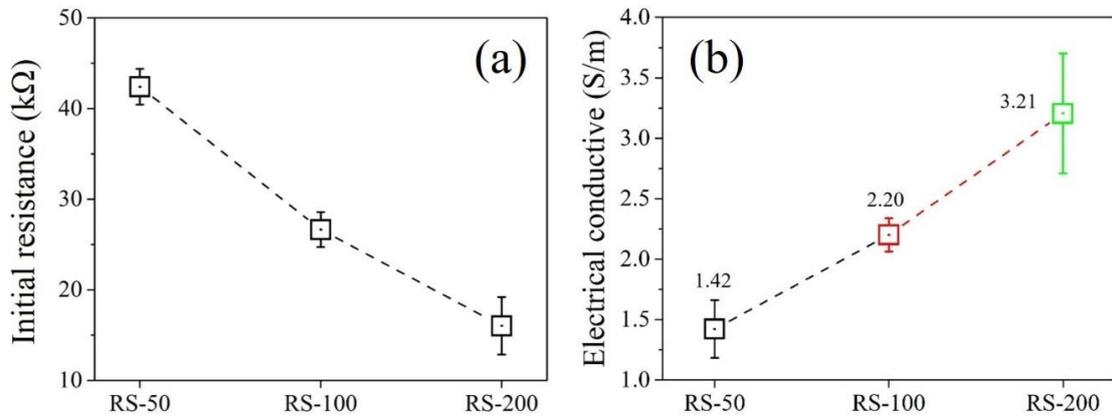
**Fig. S1** **a** Initial resistance  $R_0$  and **b** Electrical conductivity of TPU/CB strain sensors with different rotating speed
