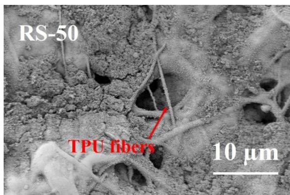
**Fig. S2** SEM images of TPU/CB strain sensor with 50 rpm
