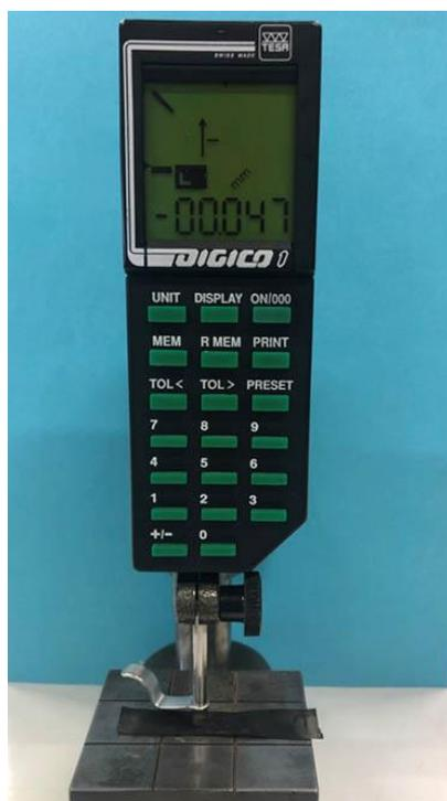
**Fig. S3** The thickness of TPU/CB strain sensor is about 50  $\mu\text{m}$
