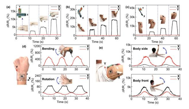
Fig. 5 Demonstration of full-range strain sensing of complex human motions by the multidirectional sensor. Detection of bending of  $\mathbf{a}$  finger,  $\mathbf{b}$  elbow, and  $\mathbf{c}$  knee joints to different degrees. Detection of multiaxial movements of  $\mathbf{d}$  wrist and  $\mathbf{e}$  shoulder joints
