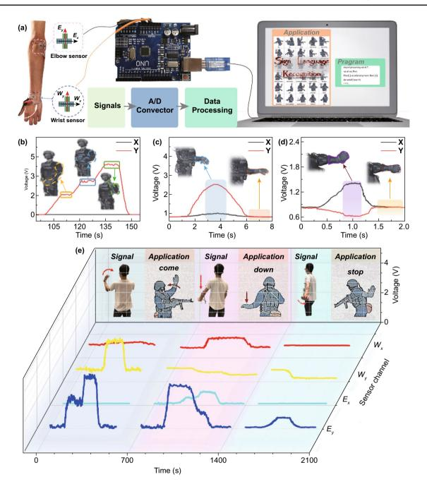
**Fig. 6** Application of the multidirectional sensor in SLRS. **a** Schematic of SLRS working principle. Manipulation of 3D character models for **b** elbow bending, **c** wrist bending, and **d** wrist rotation based on the signals generated from the multidirectional sensors attached to different parts of human body. **e** Recognition of sign languages including "come," "down," and "stop" based on the signals transmitted from four sensing channels
