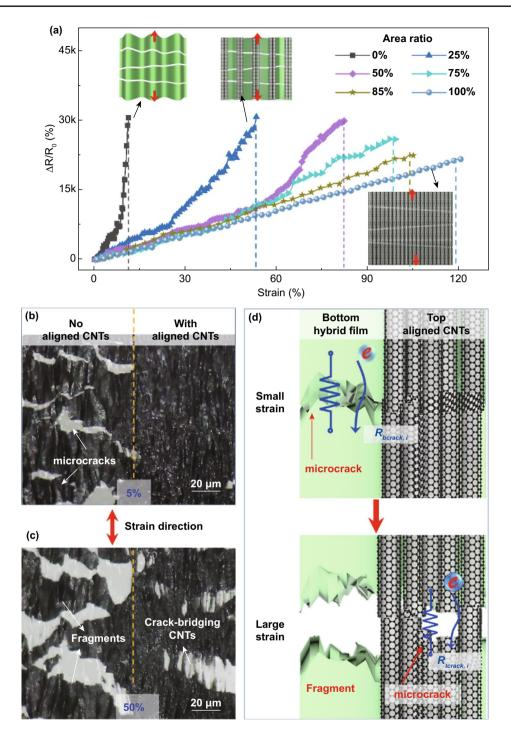
Fig. 2 Optimization of stretchability and linearity of the sensor. **a** Relative resistance changes in T-direction of bilayer sensors with different area ratios of top to bottom films: schematics of the corresponding structures in inset. Morphologies of bilayer sensors when loaded at **b** 5% and **c** 50% strains in T-direction. **d** Schematic illustration of stepwise crack propagation mechanism
