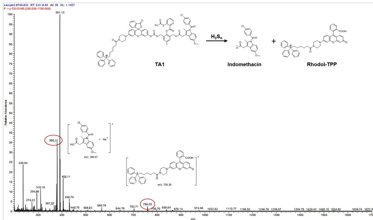
Fig. S13 ESI-MS spectrum of TA1 after incubation with Na<sub>2</sub>S<sub>3</sub> for 7 h in 10 mM PBS (pH 7.4)
