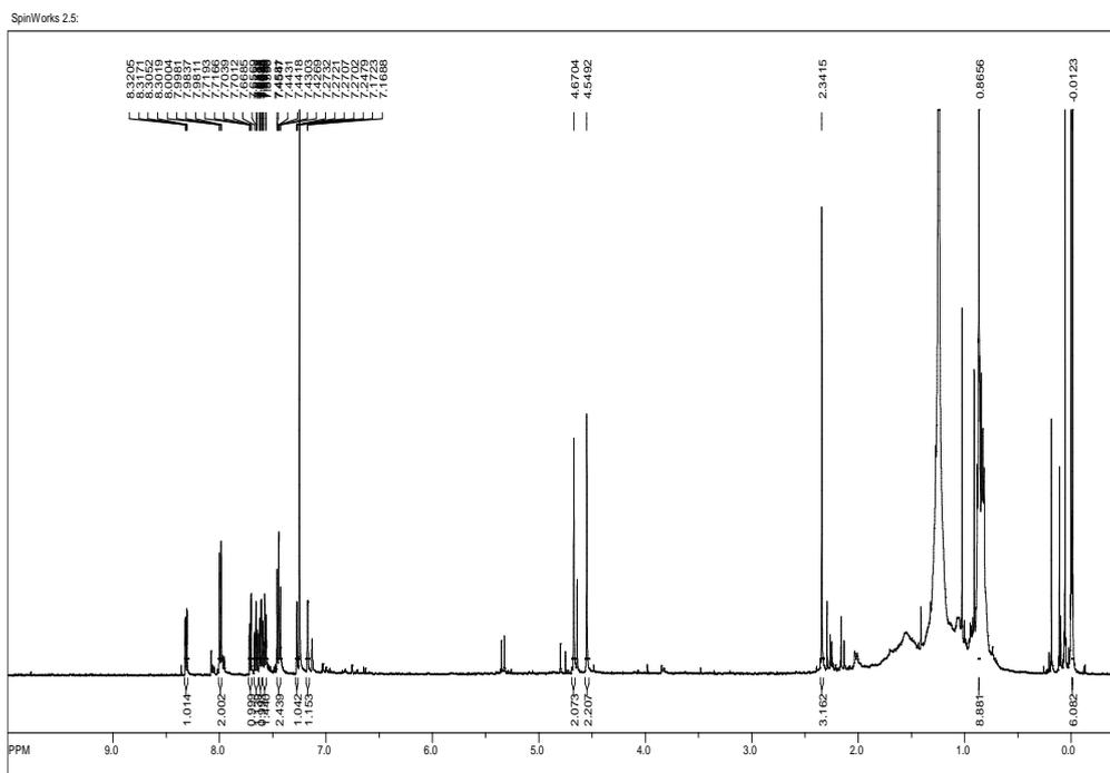
Fig. S6  $^1\text{H}$  NMR spectrum (500 MHz) of **7** in  $\text{CDCl}_3$
