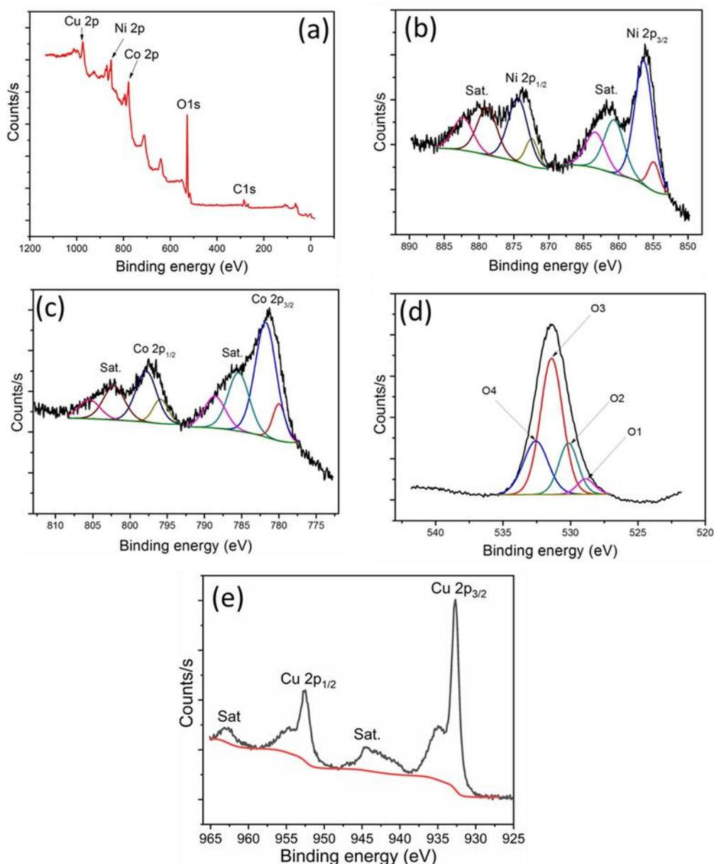
**Fig. S3** (a) The broad scan XPS spectra for the NiCo-hydroxide/NiO/CuO/Cu electrode, the narrow scan XPS spectra for the (b) Ni 2p, (c) Co 2p, (d) O 1s, and (e) Cu 2p for the NiCo-hydroxide/NiO/CuO/Cu electrode
